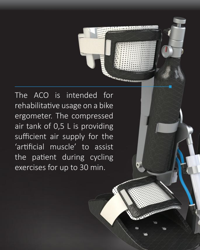
A double-acting pneumatic cylinder is the 'artificial muscle' the assist the patients muscle function and can create up to 50% of assistance during plantar- and dorsiflexion motion. The spring characteristics of the pneumatic cylinder are providing an elastic response to the movements of the human muscle.
