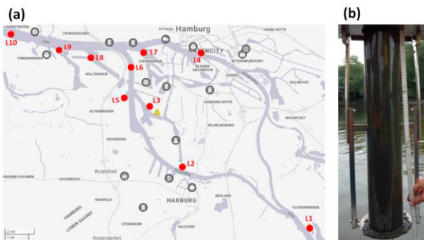
Figure 1: (a) Selected locations in the Port of Hamburg, Germany for collecting mud samples, (b) sample collector (Frahmplot).
