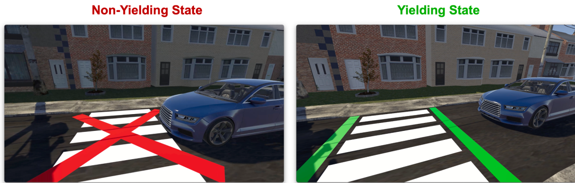
Fig. 5. Example of side-by-side image for AR concept 1, Augmented zebra crossing. Left: non-yielding state, Right: yielding state.
