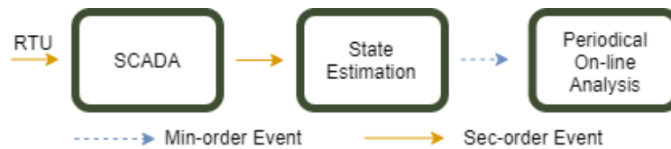
Figure A.1: The current online analysis system architecture where min-order is response time in order of minutes, and sec-order is response time in the order of seconds [37].
