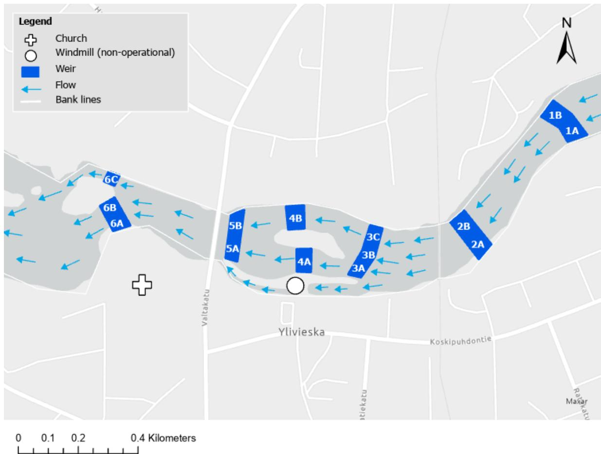
Figure 5: Schematization of hydraulic structures at Juurikoski.
