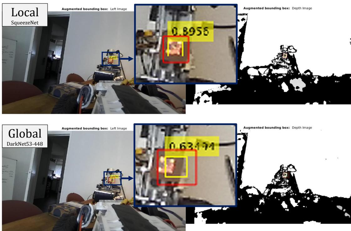
**Figure 7-9:** Detection under slight angle using a local squeezeNet and a global DarkNet53-448 based YOLOv2 detector.
