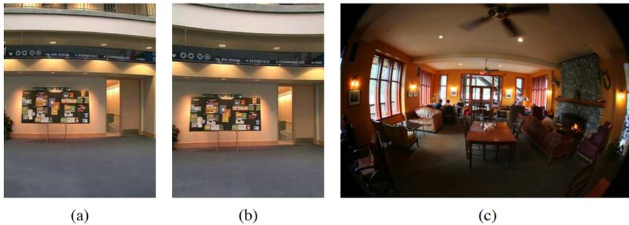
**Figure 2-2:** Three examples of lens distortion: barrel (a), pincushion (b), and fisheye (c) distortion[3].
