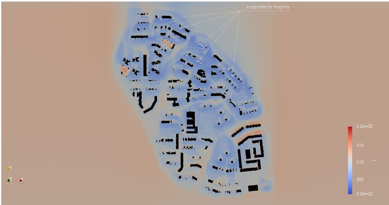
Figure 7.4: wind from S – highlighted areas with white contour [ 297.8\text{ K} < T_a \leq 305.0\text{ K} ] \Rightarrow thermally acceptable for most people; all other areas uncomfortably hot
