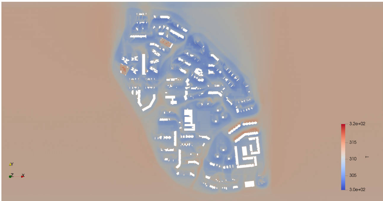
Figure 6.36: prevailing wind from South – T at pedestrian level ( z = +3.75\text{m} )
