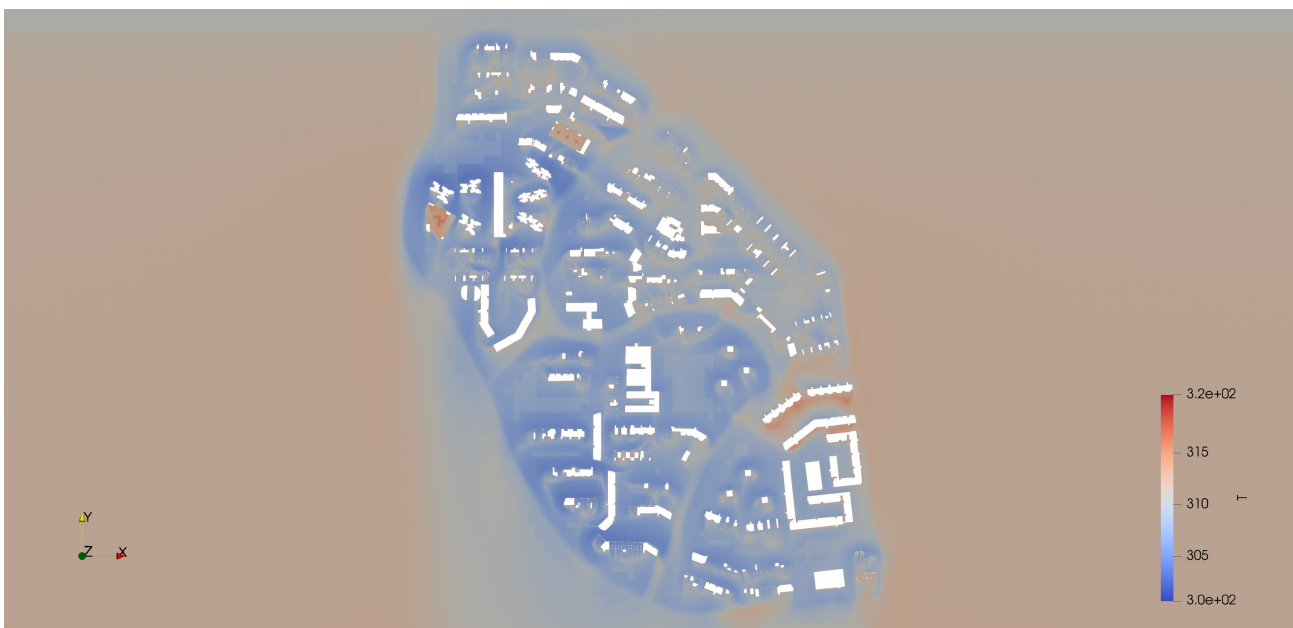
Figure 6.32: prevailing wind from North – T at pedestrian level ( z = +3.75\text{m} )
