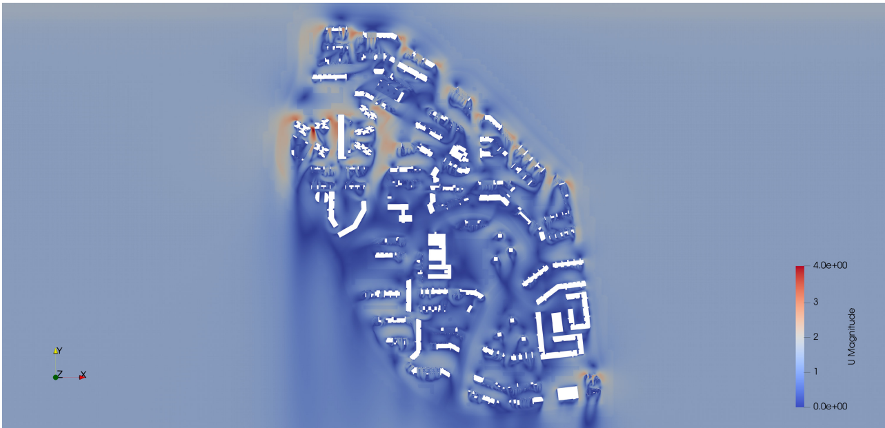
Figure 6.31: prevailing wind from North – U at pedestrian level ( z = +3.75\text{m} )
