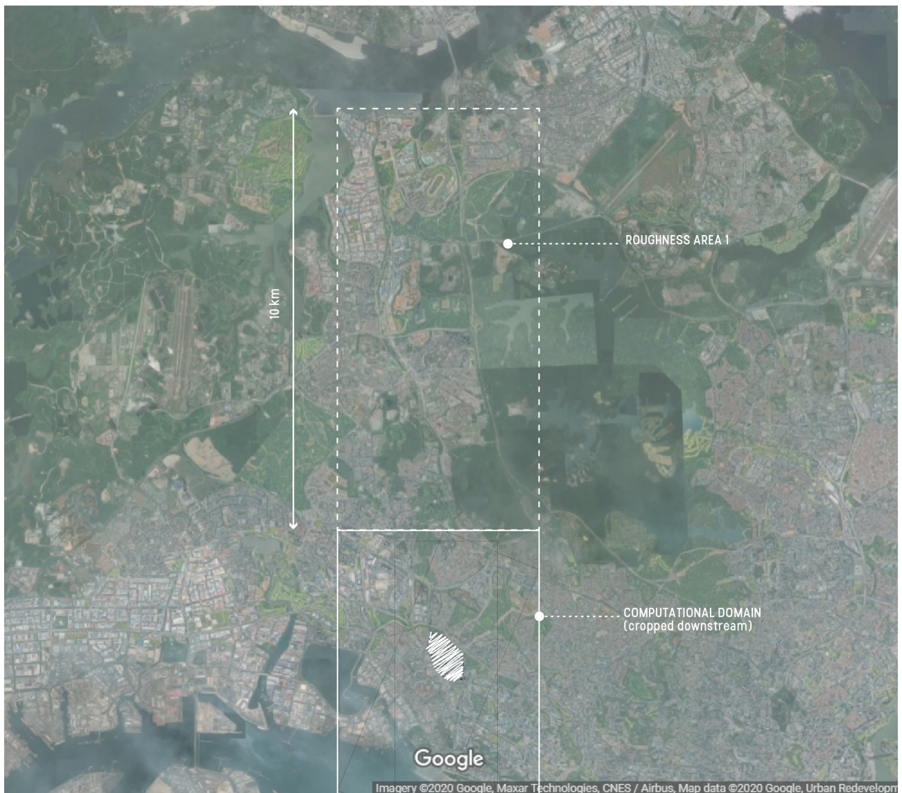
Figure 6.7: roughness area 1 (upstream of computational domain) for simulation with wind from North/North-North-east
