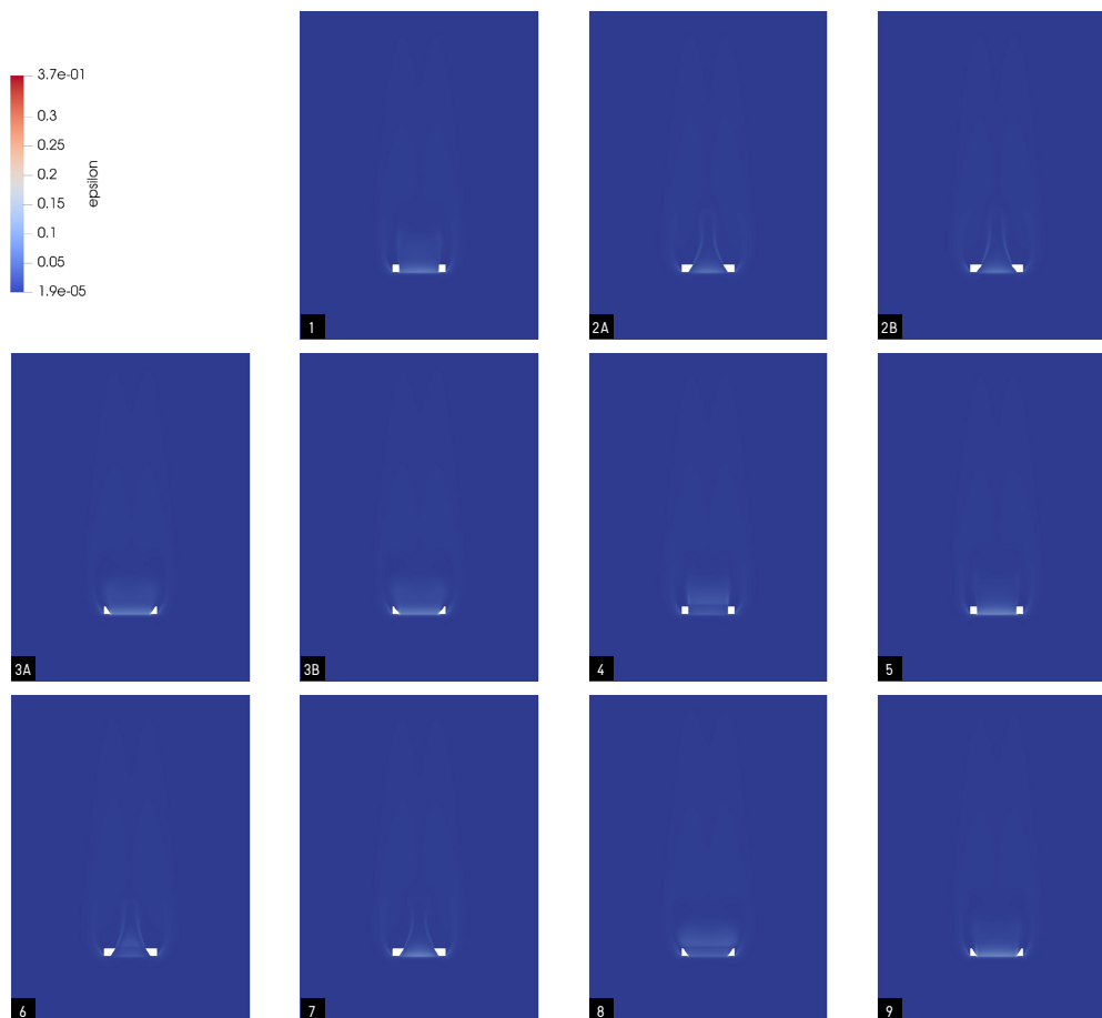
Figure 6.30: horizontal plane results for \epsilon at pedestrian level (1.75m height)
