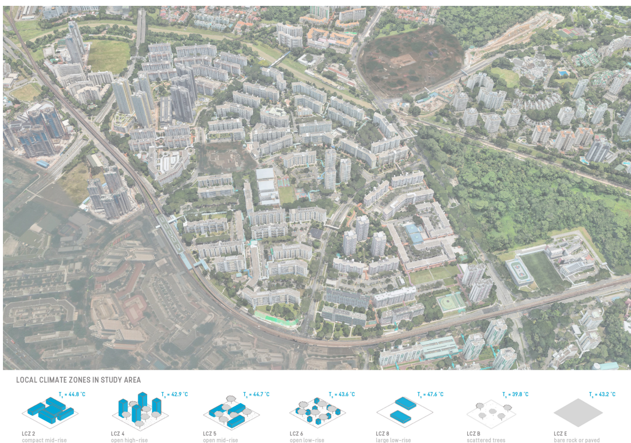
Figure 6.12: LCZs and surface temperature boundary conditions in study area
