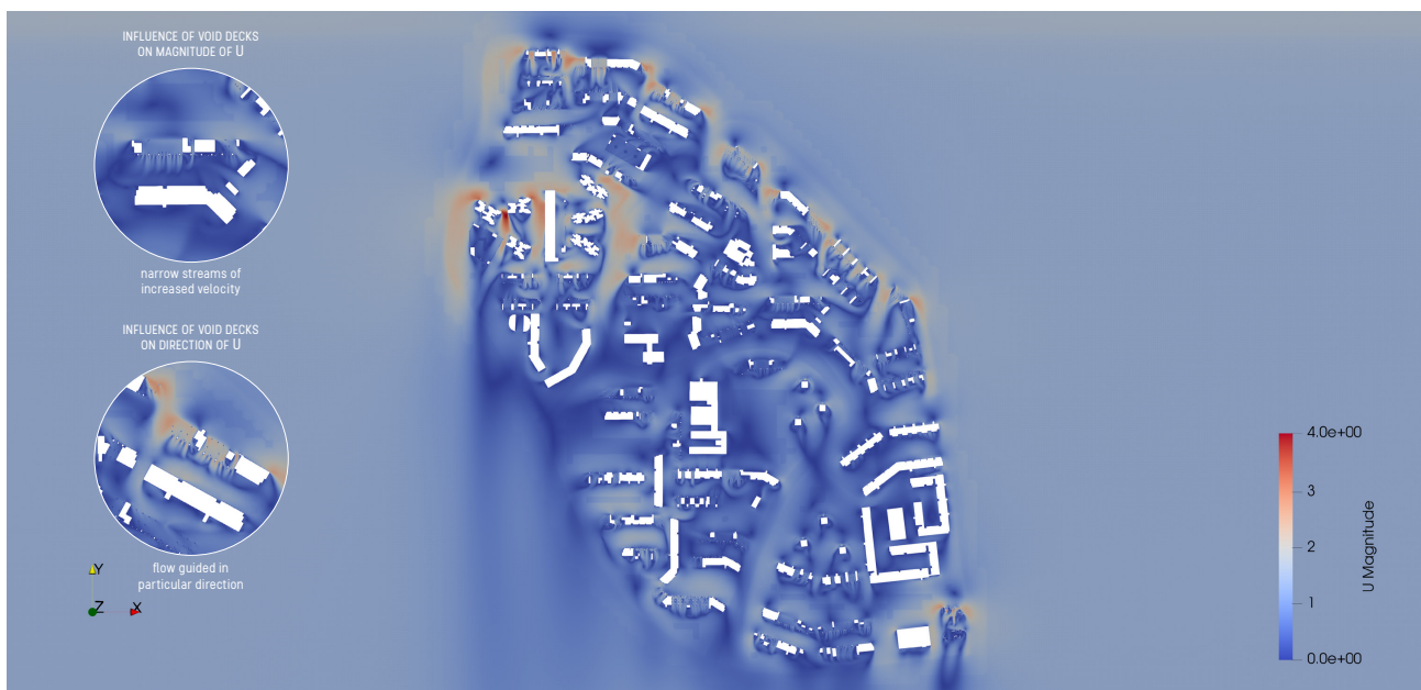
Figure 6.38: influence of void decks on magnitude and direction of U (shown for prevailing wind from North – U at pedestrian level ( z = +3.75\text{m} ))
