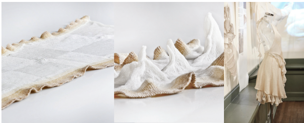
Figure 11: Jane Scott’s Programmable Knit [157, 158] emerges of the knitting machine relatively flat (left) and after exposing the knitted textile to moisture, dramatic peaks are formed (centre) (Image credit: Cristina Schek). The knitted dress (right) utilises the methods explored (Image credit: Jane Scott).
