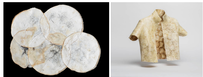
Figure 3: Moulded textile-form example. MycoTEX jacket (right) by Aniela Hoitink [70] is made from grown mycelium 'disks' (left), then bonded on a 3D mould. Image credit: MycoTEX by Aniela Hoitink.
