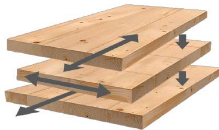
Figure 2.27: Schematic of CLT layer configuration [23]
