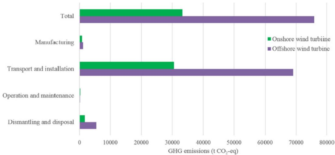
Figure 1-2: GHG emissions for onshore and offshore wind turbine [8]
