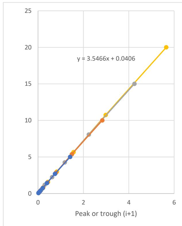
Figure 8-1: Plot of peak amplitude (i) against peak amplitude of next peak (i+1)
