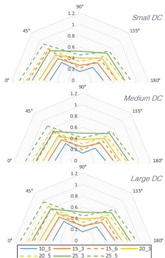
Figure 5-22: RMS absolute vertical motions [m] of the bow transfer platform
