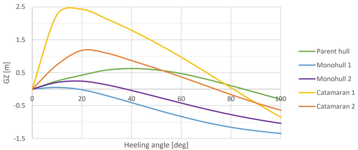
Figure 6-18: Intact stability of the parent hull and DC prototypes
