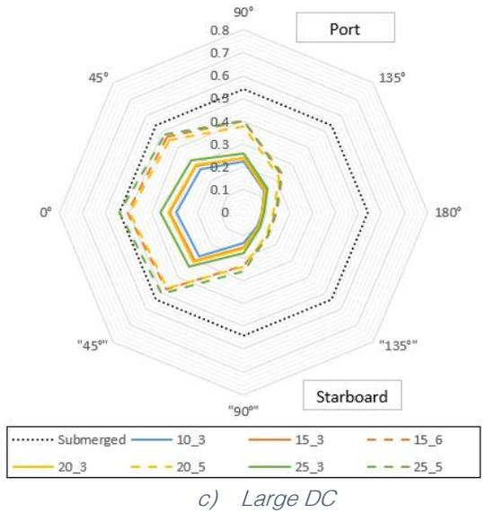
Figure 5-29: RMS relative motions [m] of the propulsor inlets
