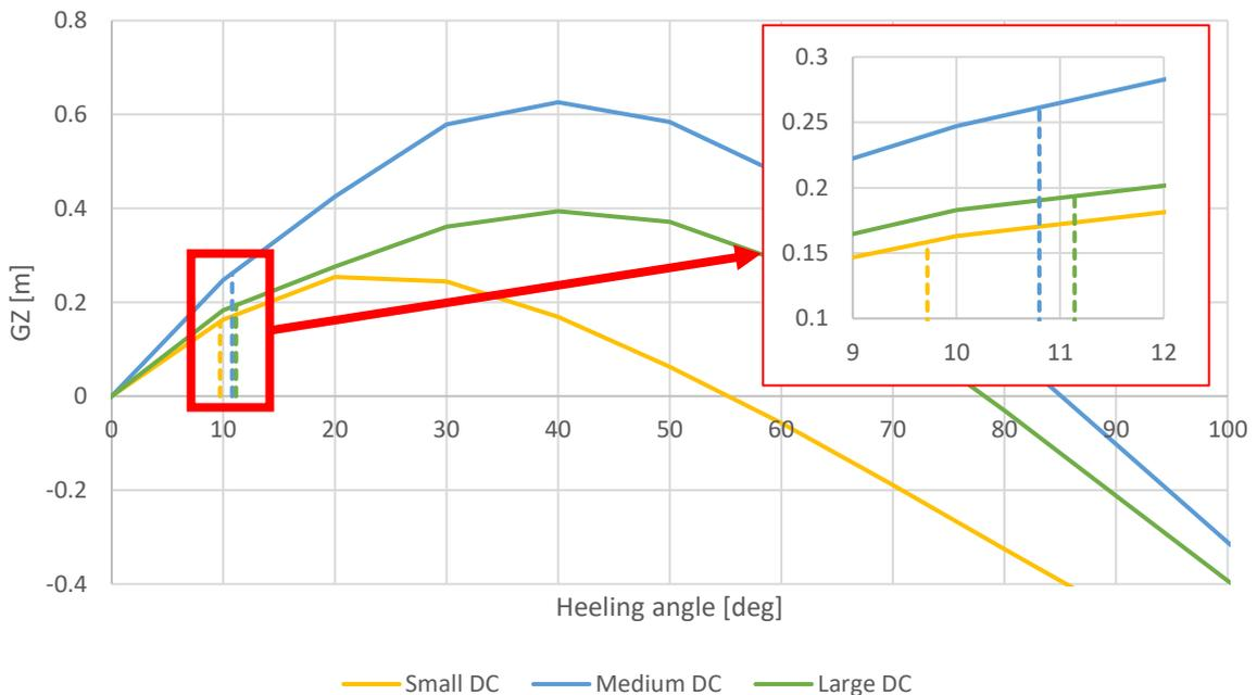
Figure D 2: Heeling angle and GZ during wave spectrum 15-3 and  $\mu = 90^\circ$
