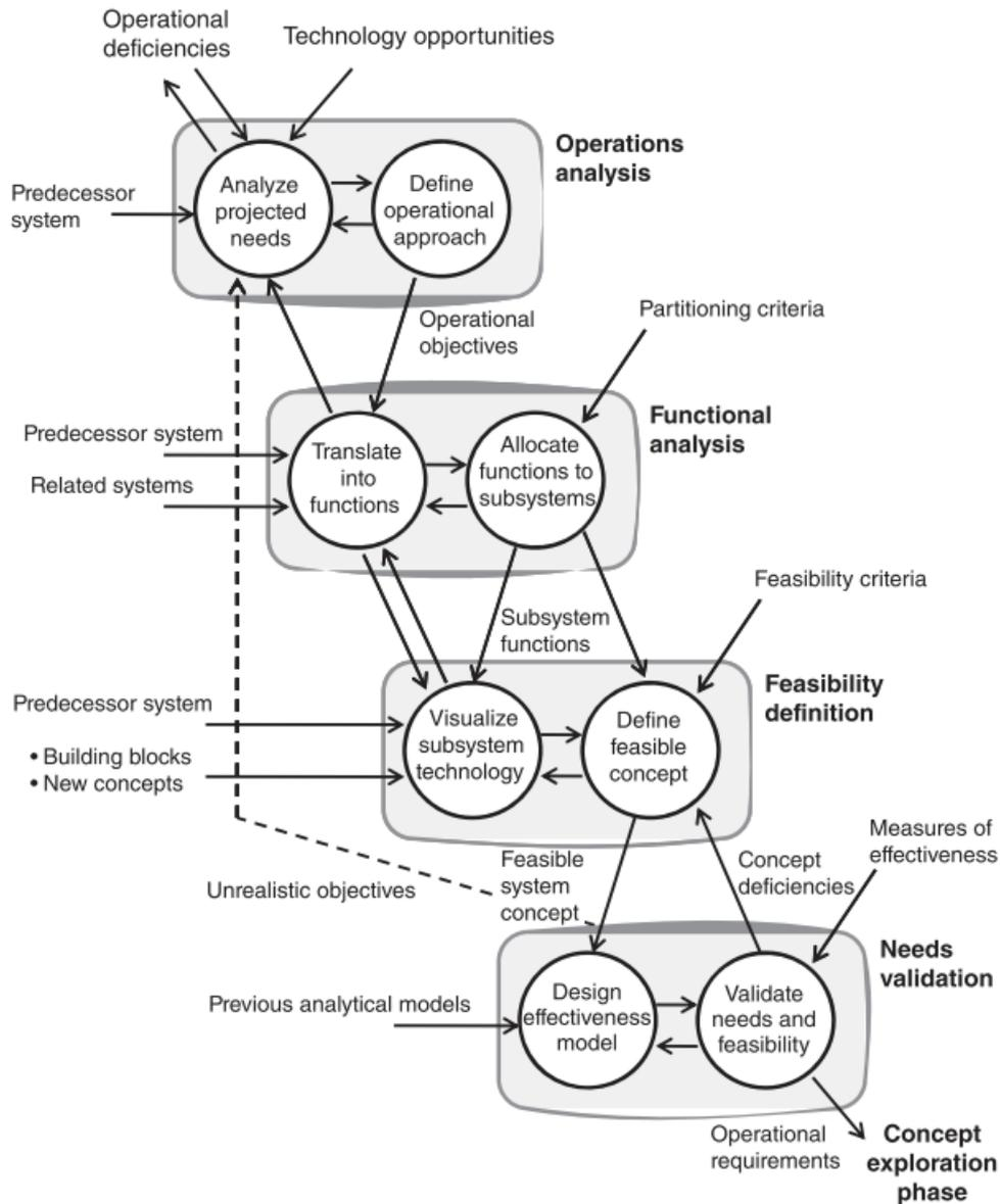
Figure 1-6: Division of the Needs analysis phase within the Systems Engineering approach [13]
