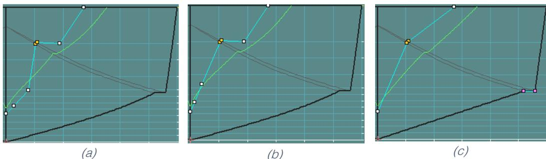
Figure 5-12: Hull made linearly stiff to obtain “flat” plates
