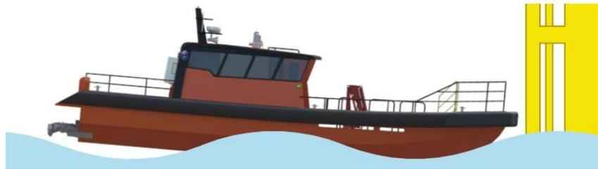
Figure 5-8: Sketched propulsor ventilation (Vessel: ProZero DCW 15 m Transfer Vessel, taken from [72])
