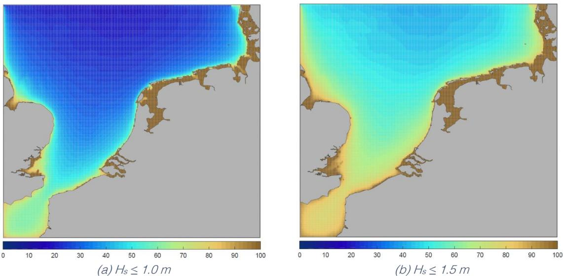
Figure 4-14: Accessibility in percentage of time, based on different thresholds [19]
