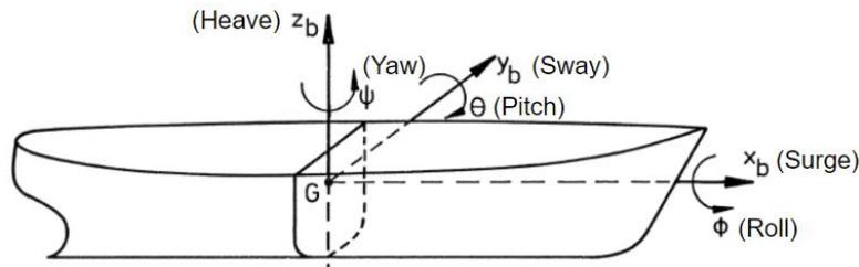
Figure 5-2: Ship motions (Adapted from [63])
