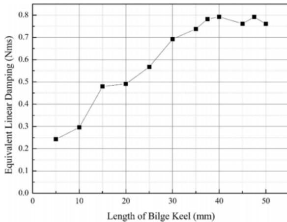
Figure 7-12: Equivalent roll damping for different bilge keel lengths [106]
