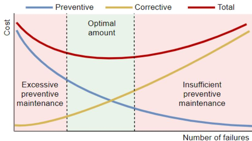
Figure 1-4: Balance between preventive and corrective maintenance (adapted from [12])
