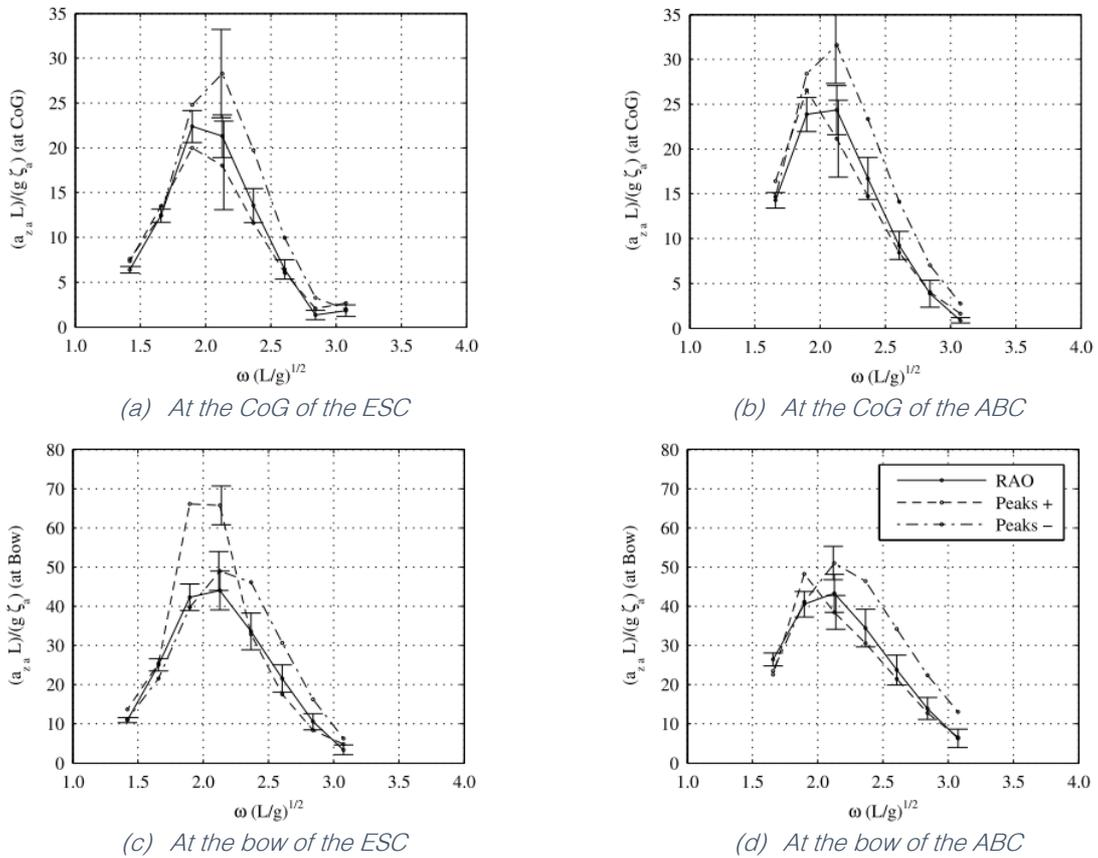
Figure 6-9: Comparison of the vertical acceleration RAOs and peaks,  $V = 25$  knots,  $\kappa = 1/30$  [66]
