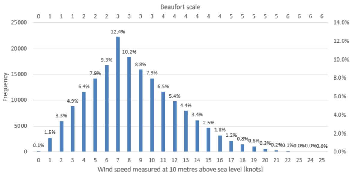
Figure 4-4: Histogram of occurring wind speeds at Hornsea One
