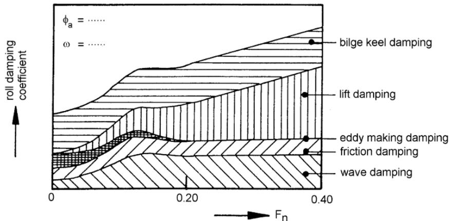
Figure 5-17: Example of roll damping components [70]
