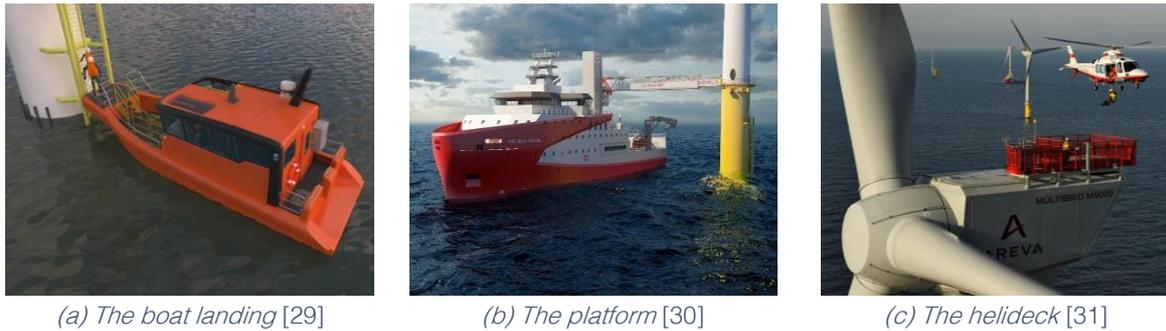
Figure 3-2: Transfer locations of offshore wind turbines
