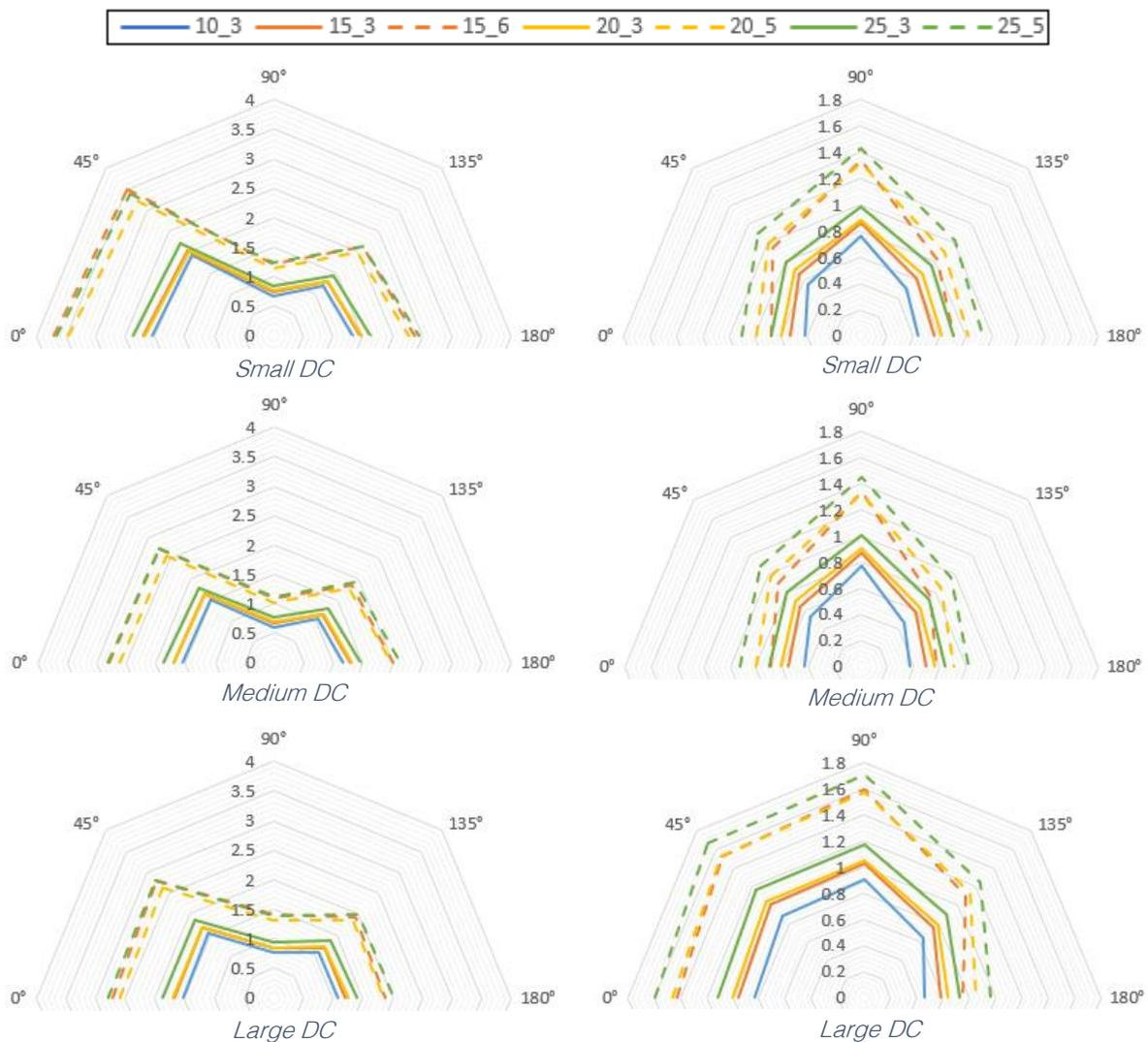
Figure 5-23: RMS absolute vertical accelerations [m/s<sup>2</sup>] at the bow transfer point
