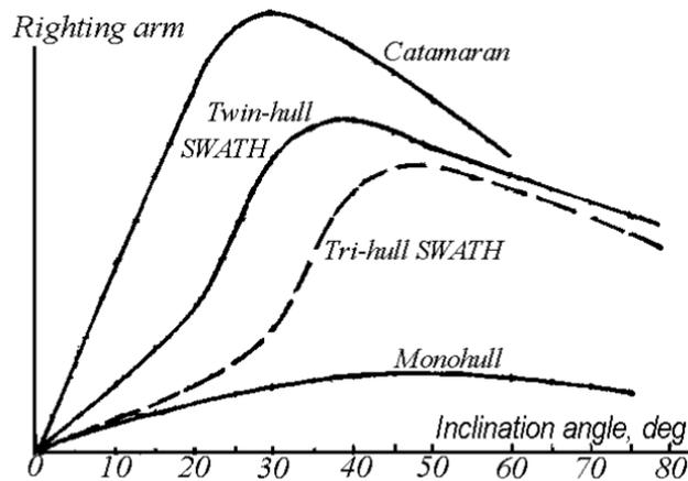
Figure 5-4: Transverse stability comparison of some multihulls and monohull [65]
