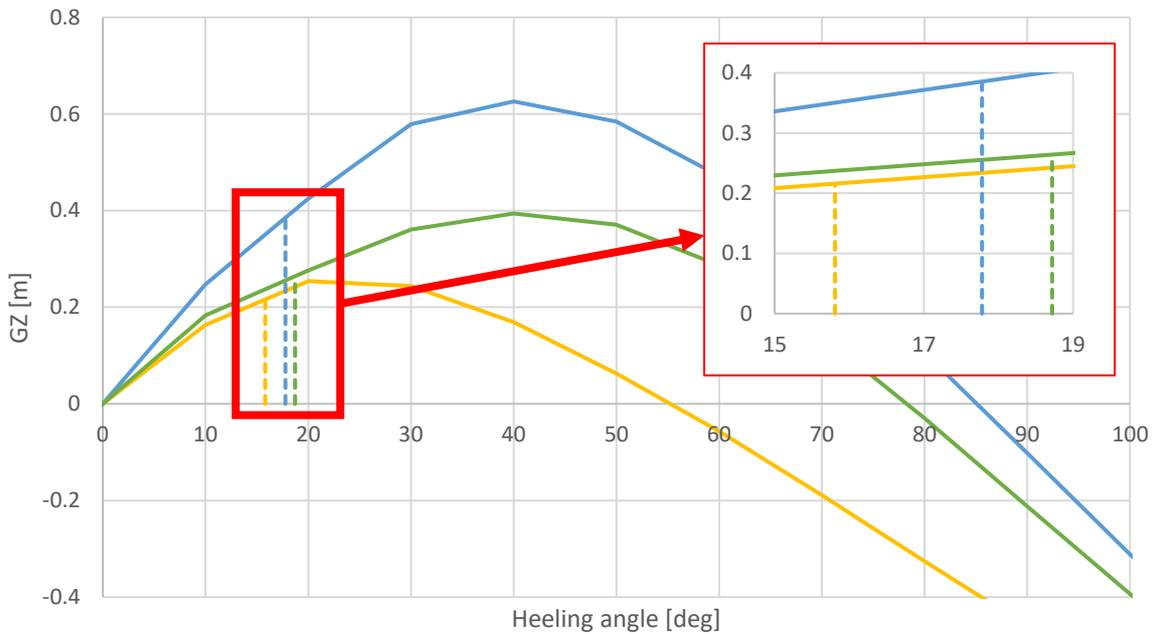
Figure D 1: Heeling angle and GZ during wave spectrum 15-6 and  $\mu = 90^\circ$
