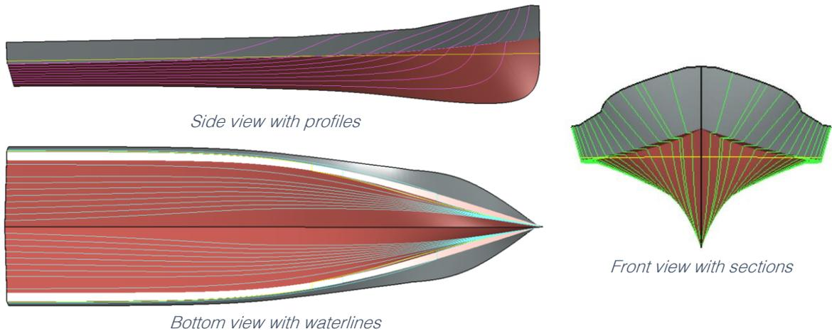
Figure 6-16: Model of "Monohull 1"
