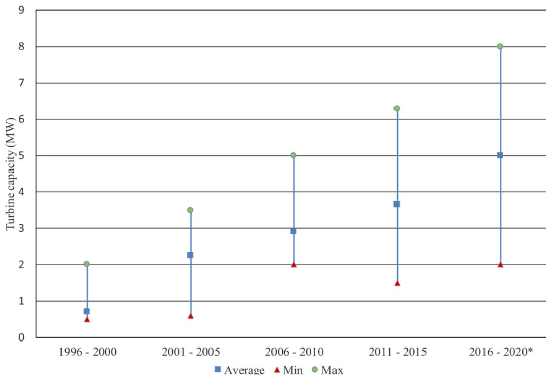
Figure 4-2: Evolution of offshore wind turbines based on the commissioning period. The last period involves the projects in pre/under construction. [44]
