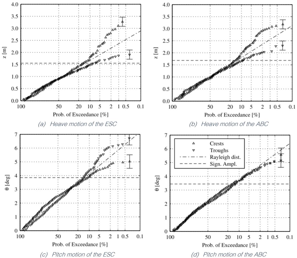
Figure E 2: Rayleigh plots of ship motions,  $H_s = 3.5$  m,  $V = 35$  knots [66]
