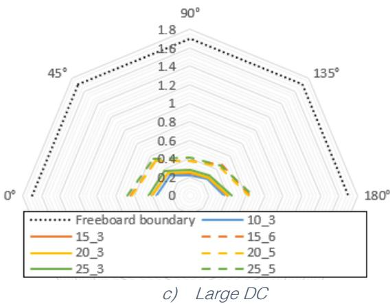
Figure 5-28: RMS relative motions [m] of the bow transfer point
