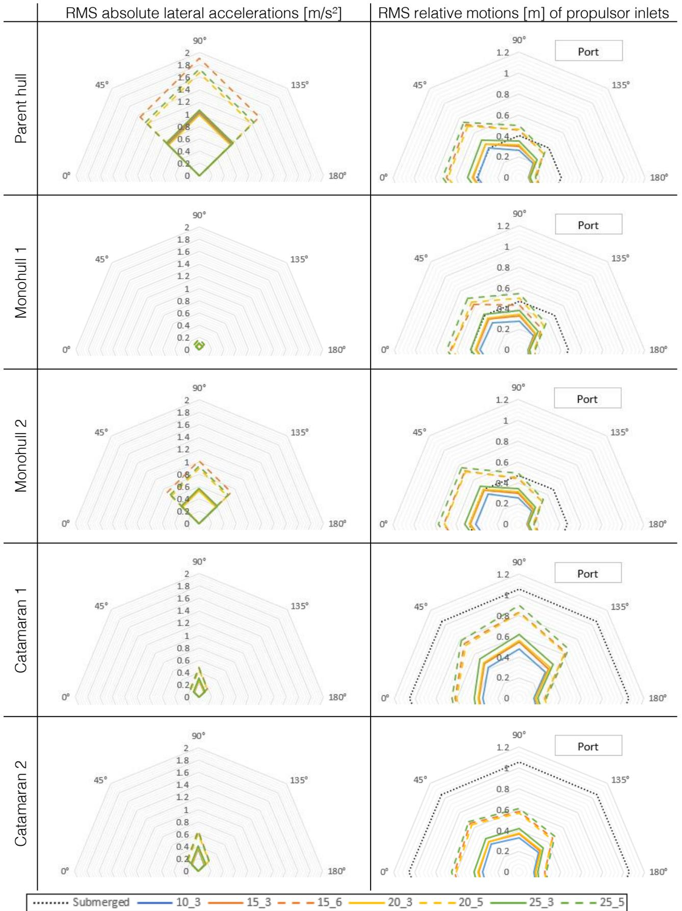
Figure 7-8: Comparison of lateral accelerations at the bow and relative motions of propulsor inlets
