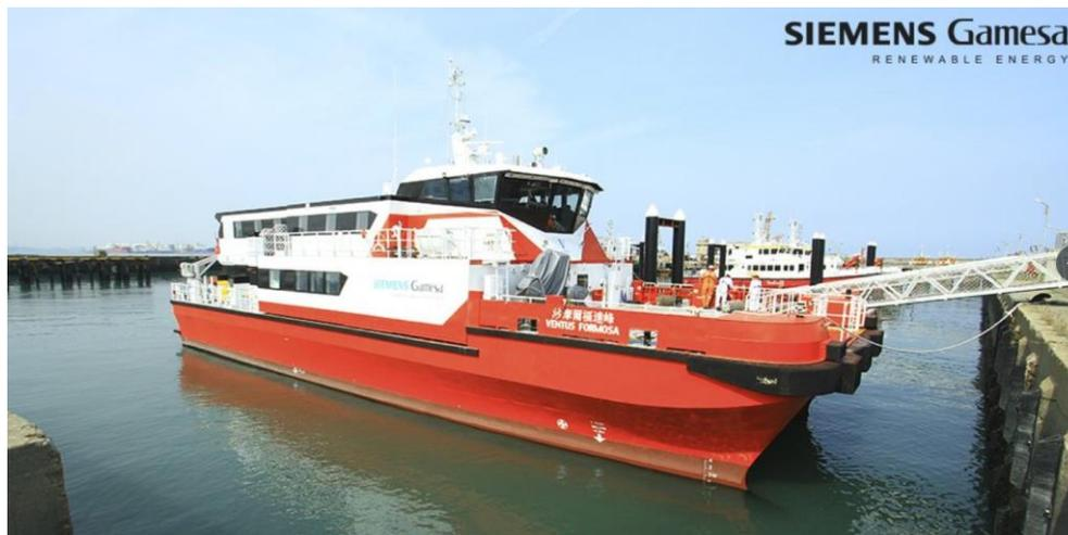
Figure 3-7: Purpose-built Service Accommodation and Transfer Vessel deployed by Siemens Gamesa [39]
