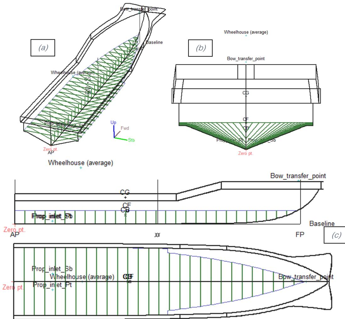
Figure 5-15: (a) Perspective, (b) section, (c) profile and (d) bottom view of large DC with input parameters
