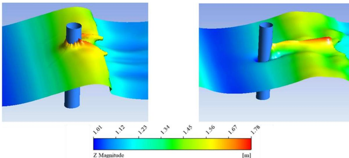
Figure 4-10: Breaking wave flow around the monopile foundation [55]
