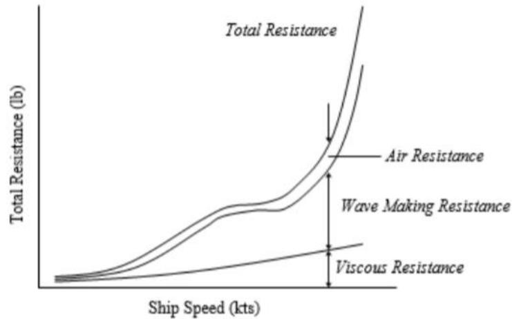
Figure 4-5: Components of hull resistance [49]
