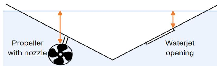
Figure 5-27: Propulsors and the depth to their inlet
