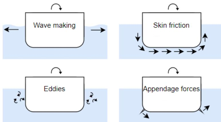
Figure 5-18: Illustration of viscous roll damping sources at zero-speed (adapted from [77])
