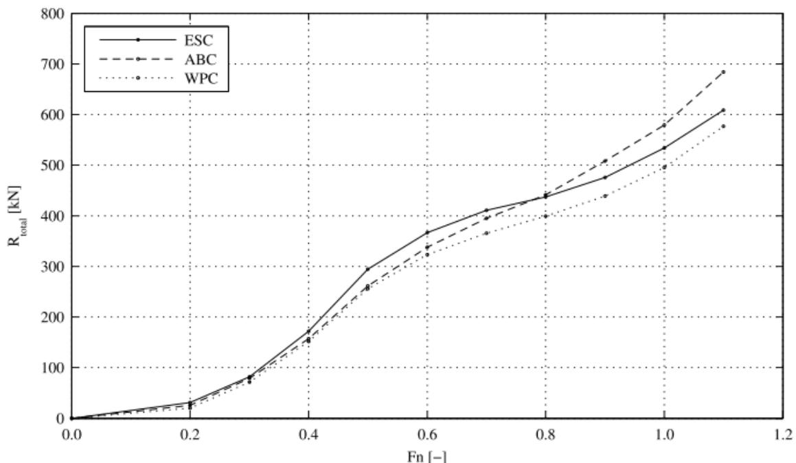
Figure E 1: Calm water total resistance of the parent hull (ESC) and the ABC [66]
