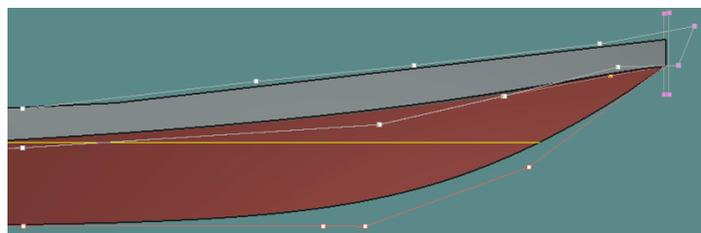
Figure 5-11: Profile view of altered bow shape and hard chine height
