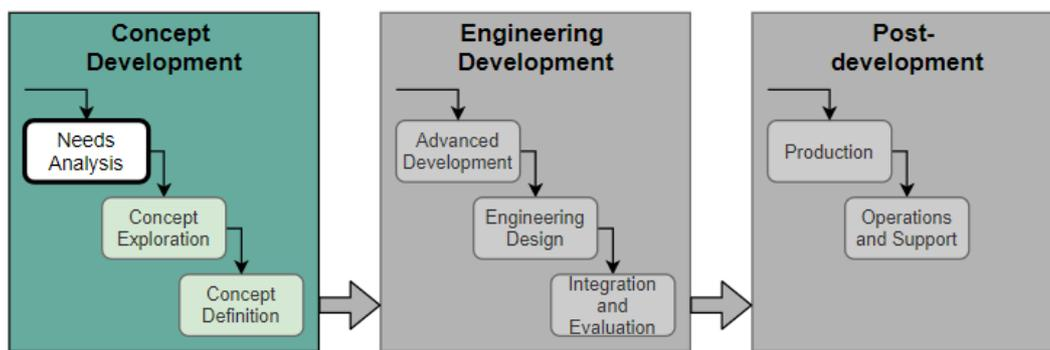
Figure 1-5: Systems engineering lifecycle model (Adapted from [13])
