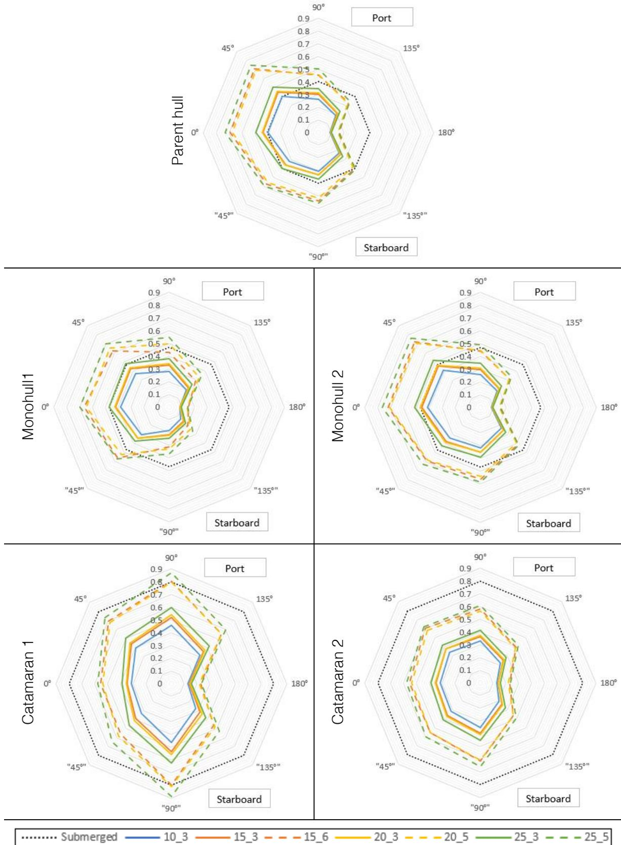
Figure H 3: RMS relative motions [m] of propulsor inlets
