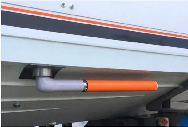
Figure 7-14: RotorSwing Magnus stabiliser [110]
