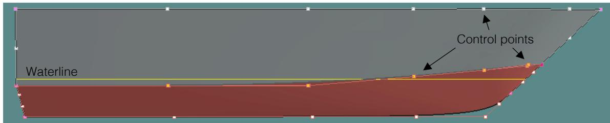
Figure 5-10: Default hull shape of workboat by MAXSURF Modeler
