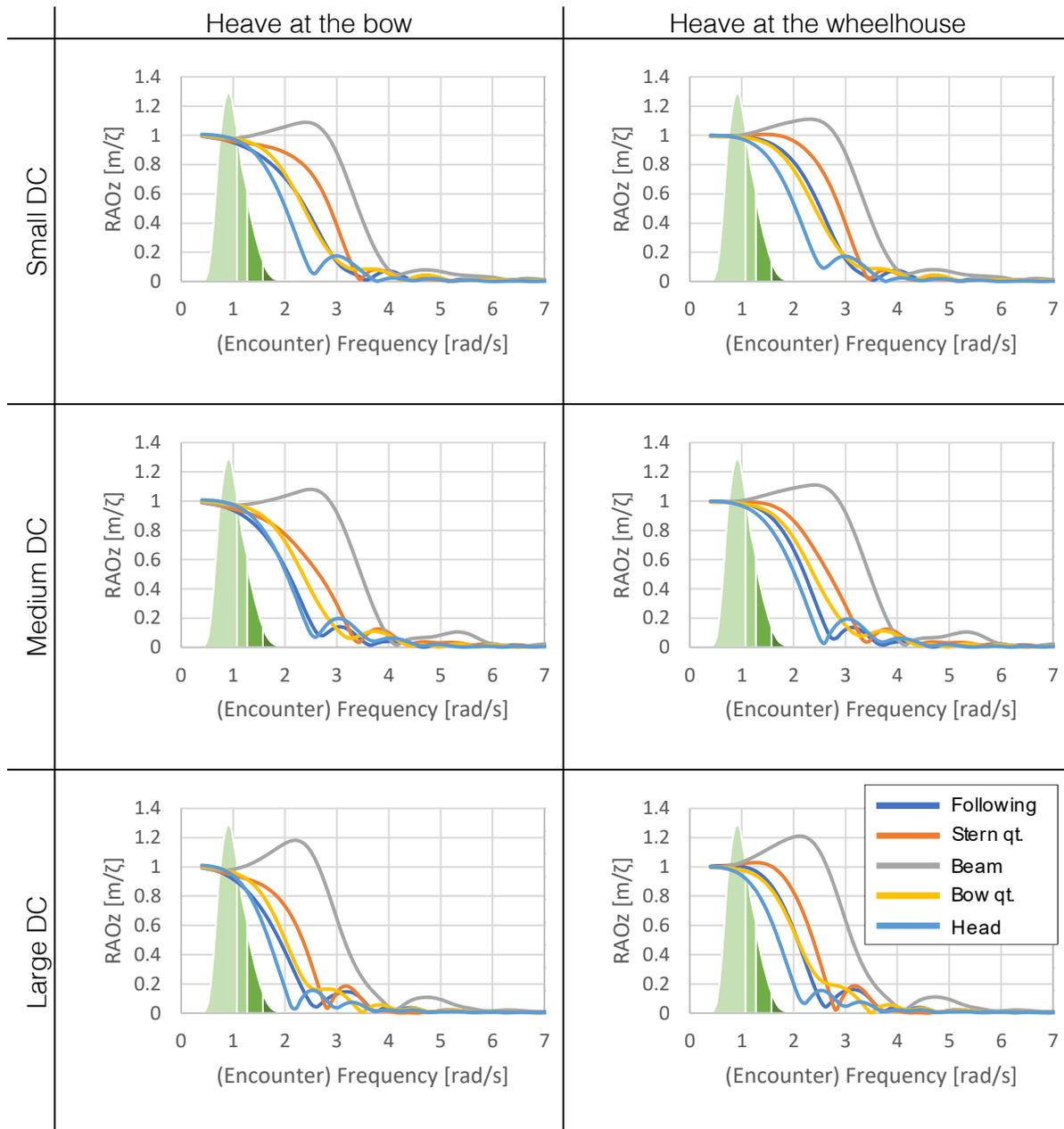
Figure 5-20: Heave RAOs at the bow transfer point and the wheelhouse
