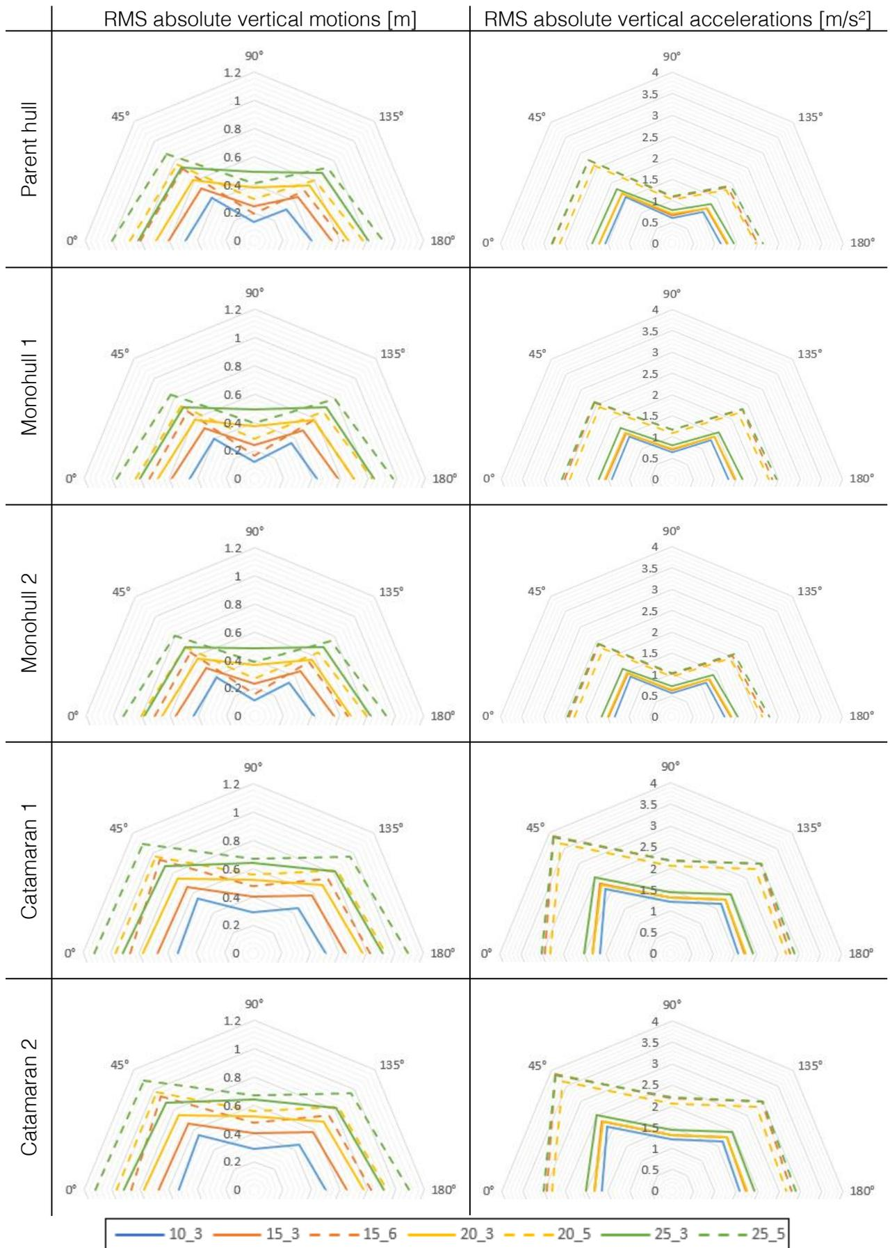
Figure 7-7: Comparison of vertical motions and accelerations at the bow transfer point
