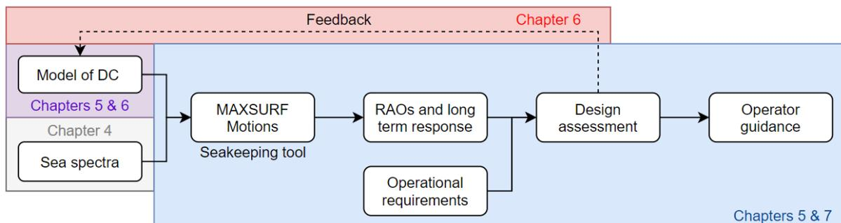
Figure 5-9: Seakeeping performance analysis method (Adapted from [59])
