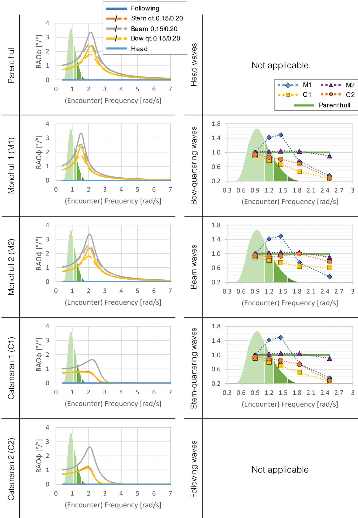
Figure 7-3: Roll RAOs at the bow and wheelhouse
