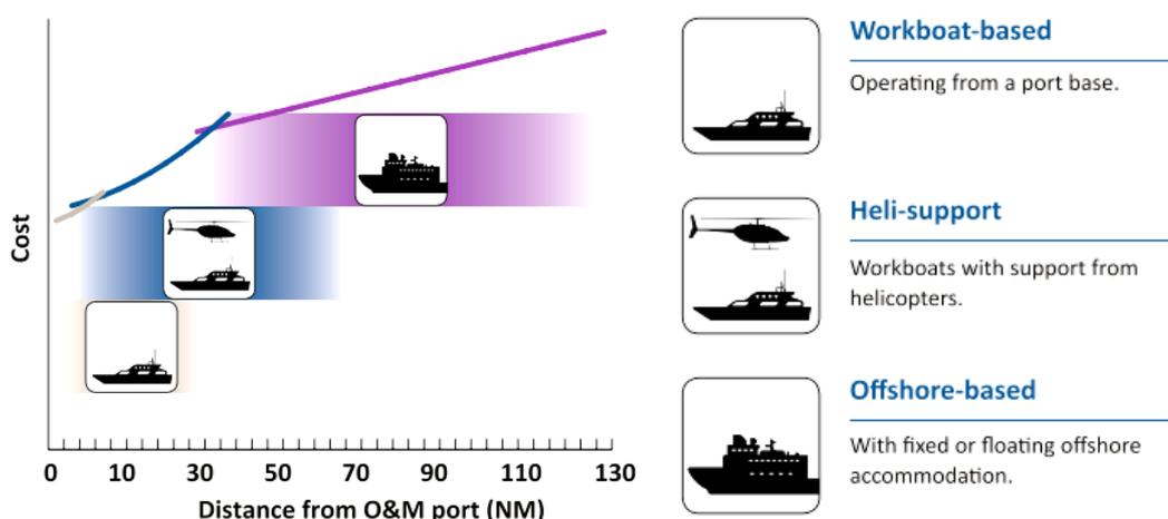
Figure 4-1: Lowest cost O&M strategy as a function of distance from O&M port [2]
