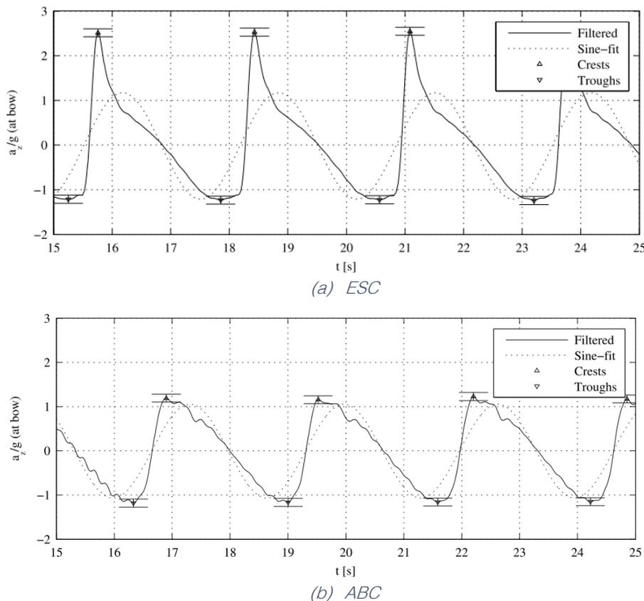
Figure 6-10: Time trace of the vertical acceleration level measured at the bow
