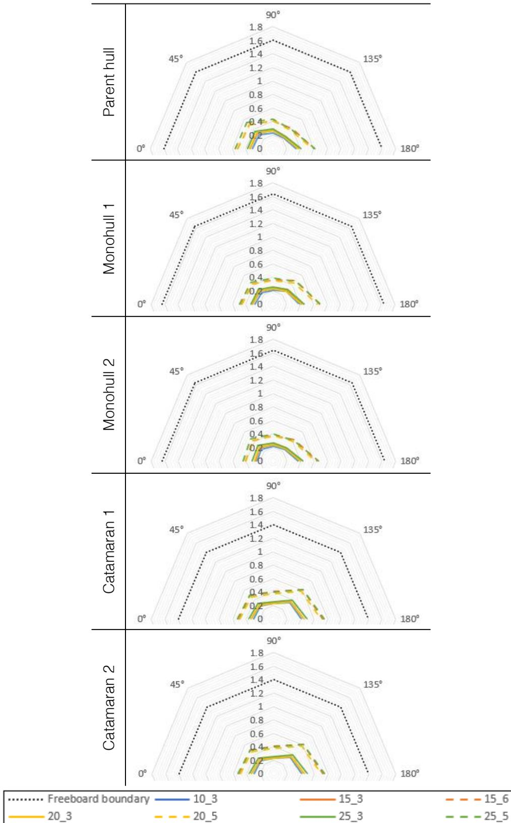
Figure H 2: RMS relative motions [m] of the bow transfer point
