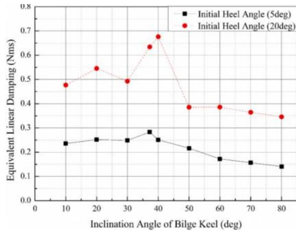
Figure 7-13: Equivalent roll damping for bilge keels of different installation orientations [106]
