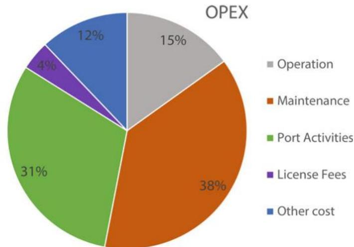
Figure 2-2: Breakdown of OPEX of an offshore wind farm [17]
