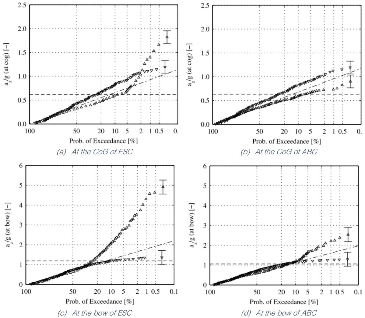
Figure E-3: Rayleigh plots of vertical accelerations,  $H_s = 3.5$  m,  $V = 35$  knots [66]
