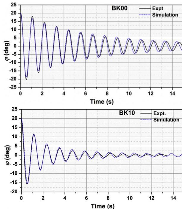
Figure 7-11: Comparison of measured and simulated free roll decay for  $\varphi_0 = 20^\circ$  [99]
