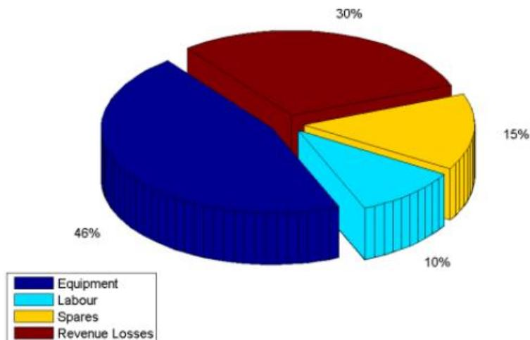
Figure 2-3: Breakdown of wind farm unplanned corrective maintenance costs [25]
