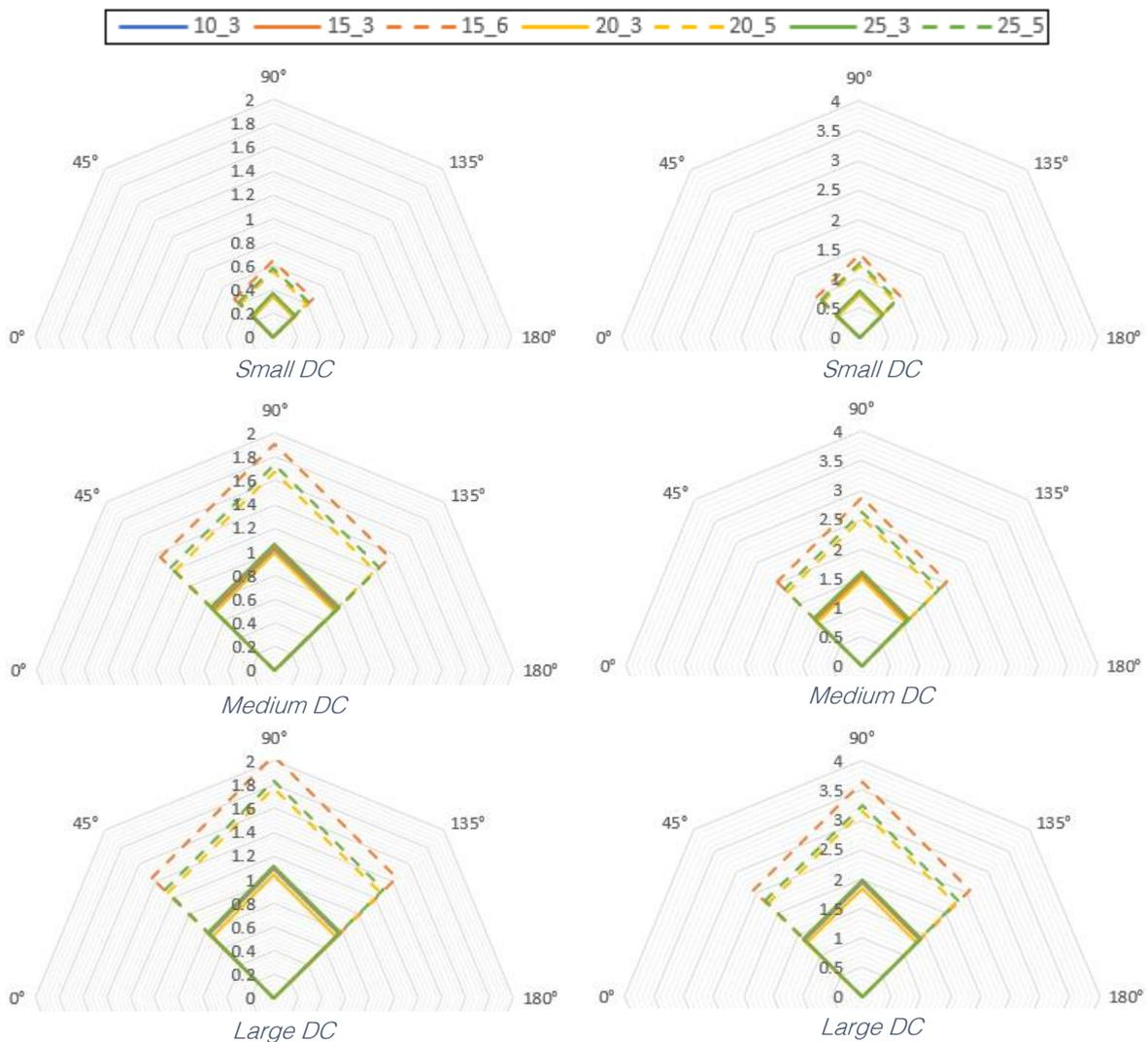
Figure 5-25: RMS absolute lateral acceleration [ $m/s^2$ ] due to roll at the bow transfer point
