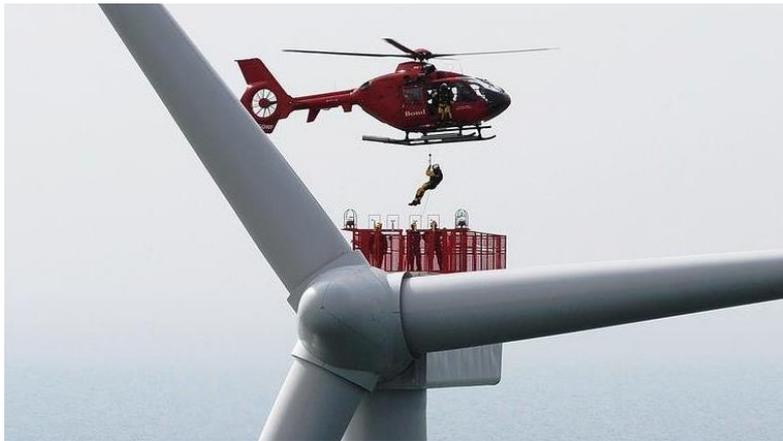
*Figure 3-8: Helicopter transferring a technician to the heli-hoist platform [41]*
