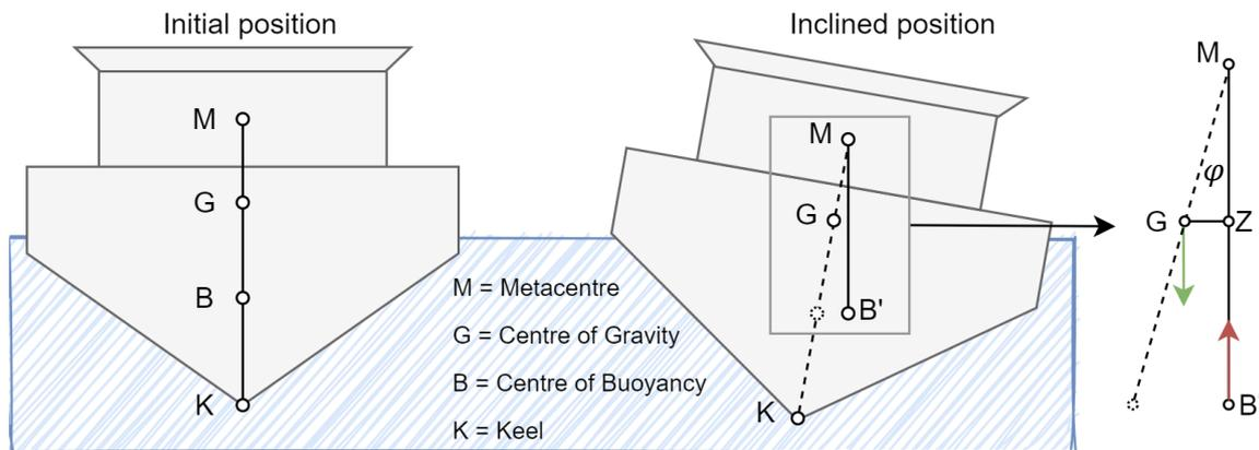
Figure 5-3: Ship transverse stability
