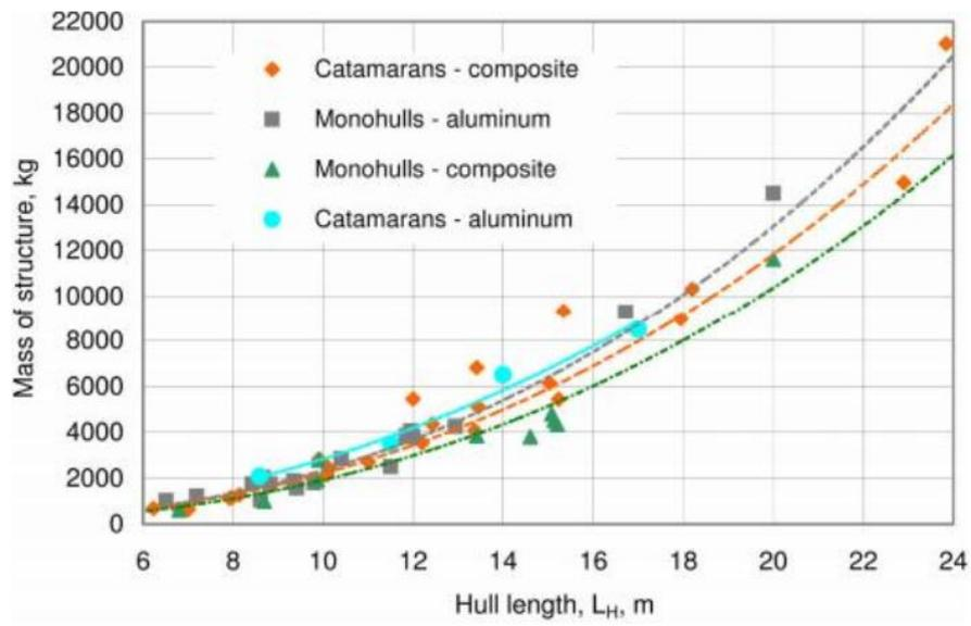
Figure 7-18: Data on structure mass for catamarans and monohulls built with composite and aluminium [100]
