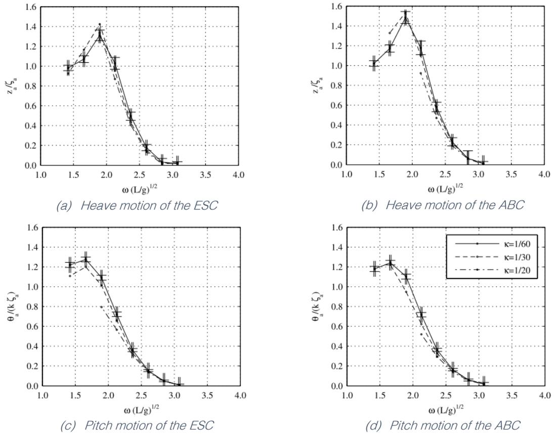
Figure 6-8: Comparison of the RAOs and their dependence on the wave steepness,  $V = 25$  knots [66]
