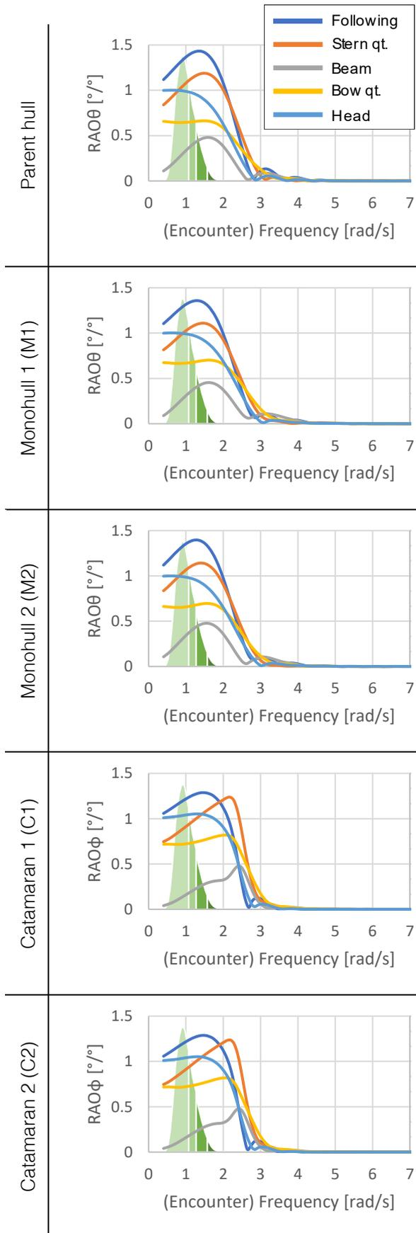
Figure 7-5: Pitch RAOs at the bow and wheelhouse
