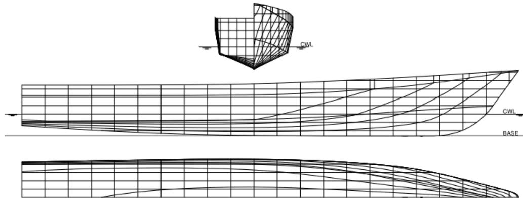
(a) Parent hull with a conventional bow
