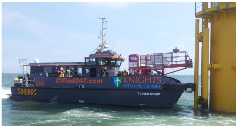
Figure 3-5: Crew Transfer Vessel with Turbine Access System [36]
