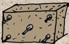
Typha pressed panel directly on facade
