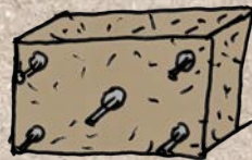
Typha pressed panel directly on facade
