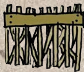
Reed clamped by wooden slat
