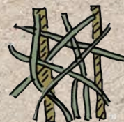
Willow withies randomly nailed on substructure
