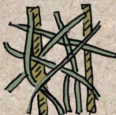
Willow withies randomly nailed on substructure
