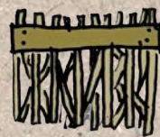
Reed clamped by wooden slat
