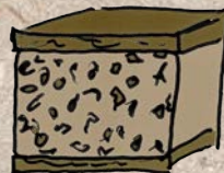
Typha pressed panel be- tween frame
