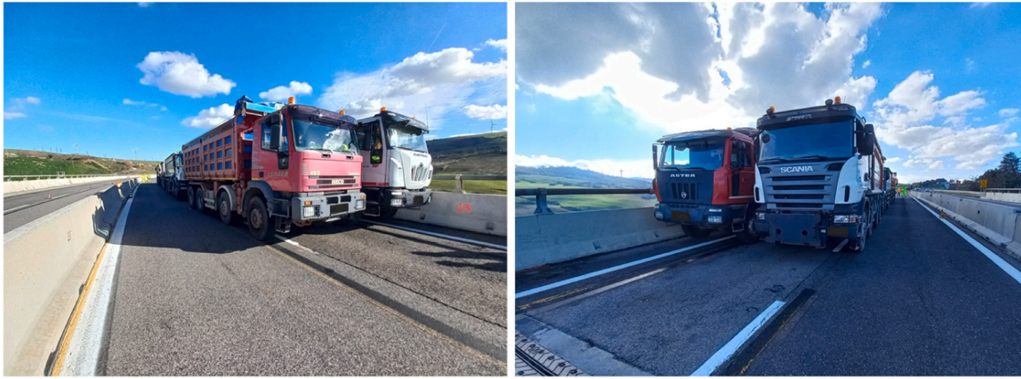
Fig. 18. Execution of the PLT on the case study bridge.
