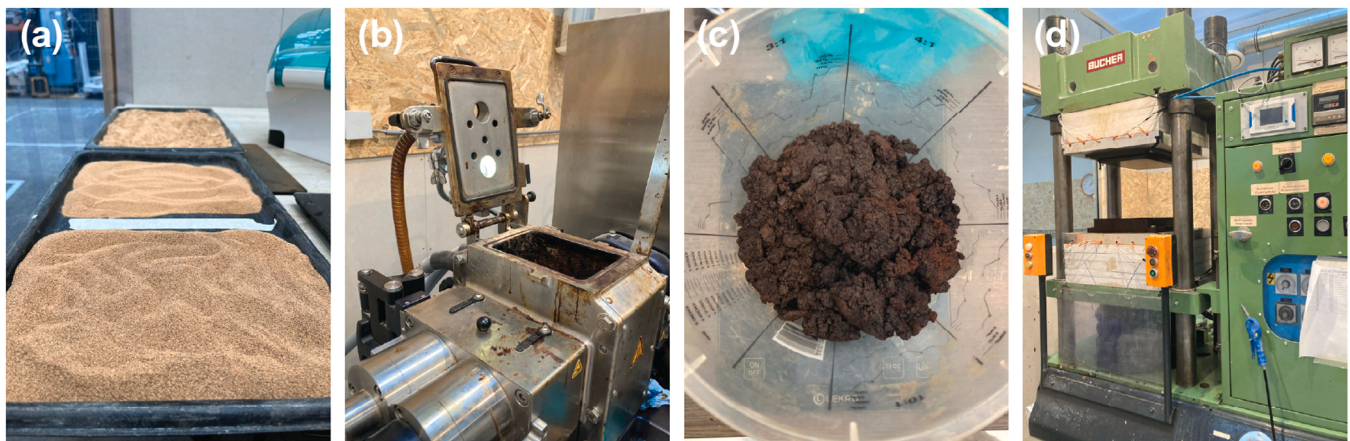
Fig. 3. (a) Milled and sieved walnut shell filler; (b) open kneader; (c) bulk moulding compound pre-pressing; (d) hydraulic press.
