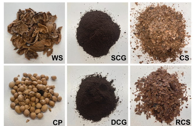
Fig. 2. Raw filler material as received, SCG and DCG dried.
