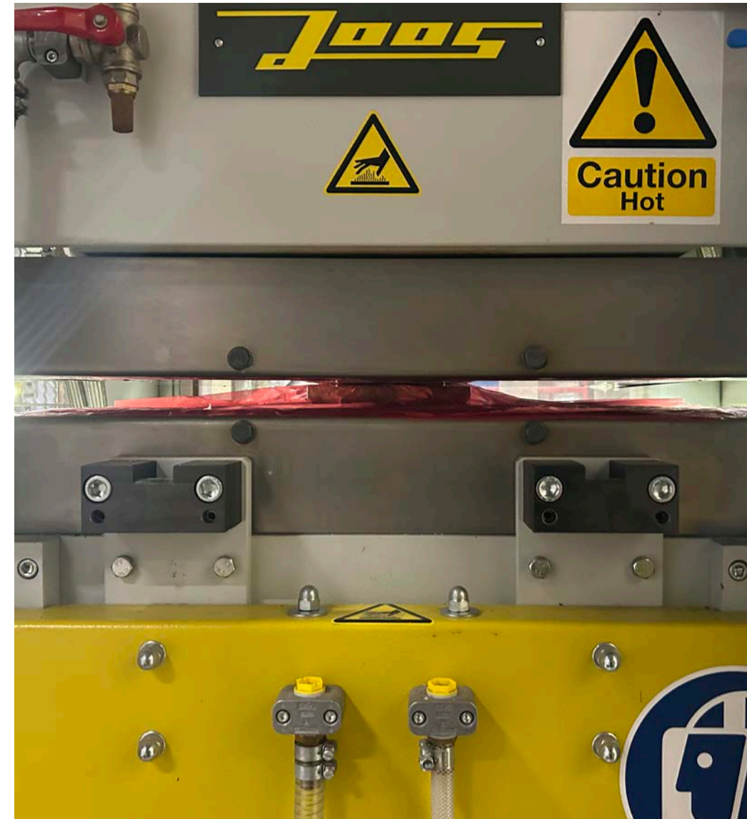
Hot-pressing at specific conditions (time, pressure, temperature).
