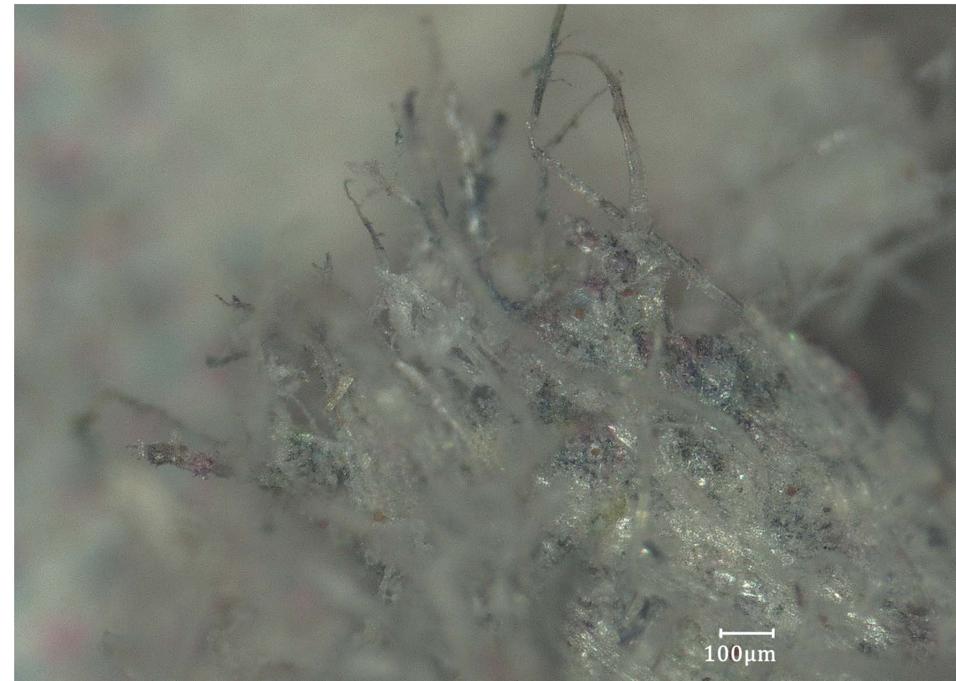
Shredded and untreated newspaper fibres x150 magnification
