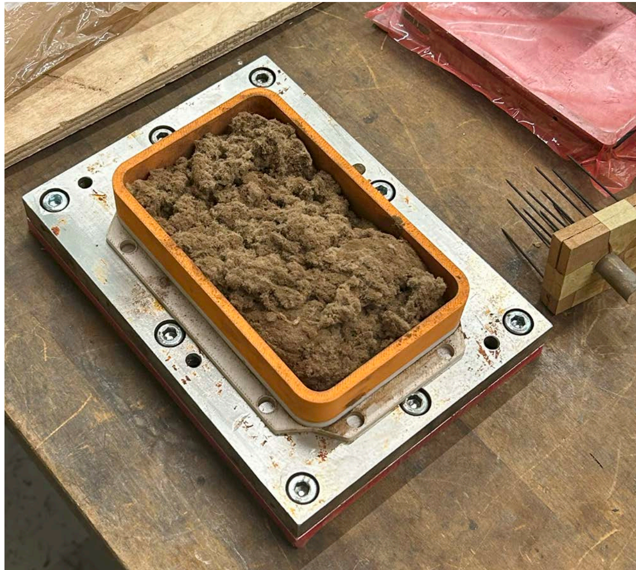
Preparing mixture in mould using the funnel and mixing tool.
