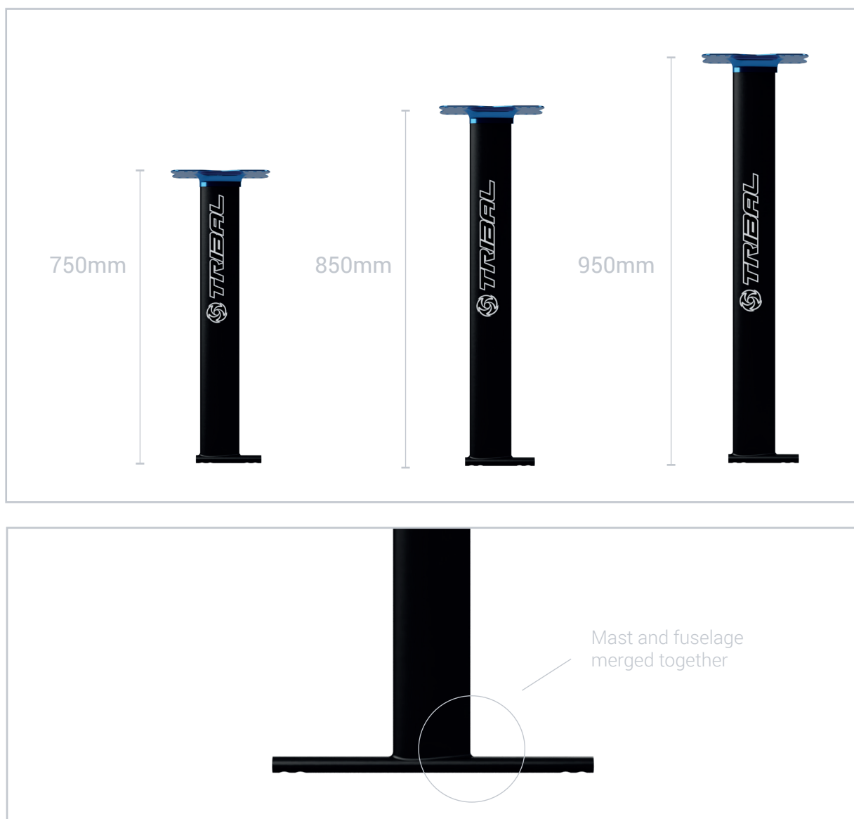
Figure 31. Top; different mast sizes, below; merged result
