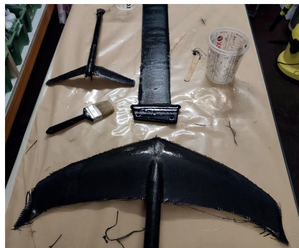
Figure 97. Hand laminating carbonfiber
