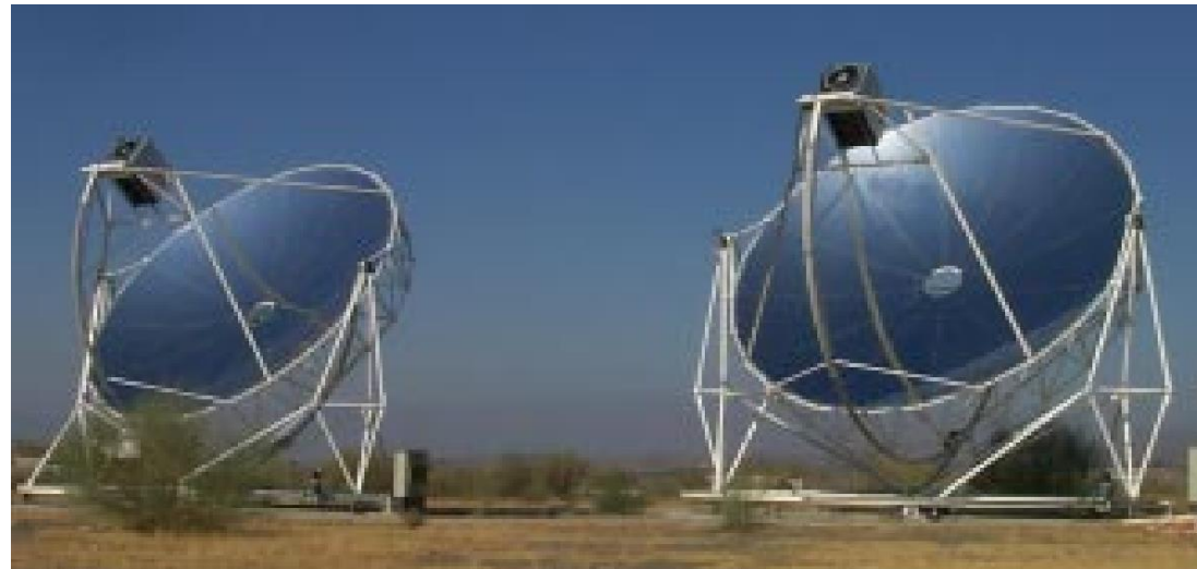
Figure C11: Two 10-kW SBP Eurodish prototypes at Plataforma Solar de Almería, Spain (Mancini et al., 2003).
