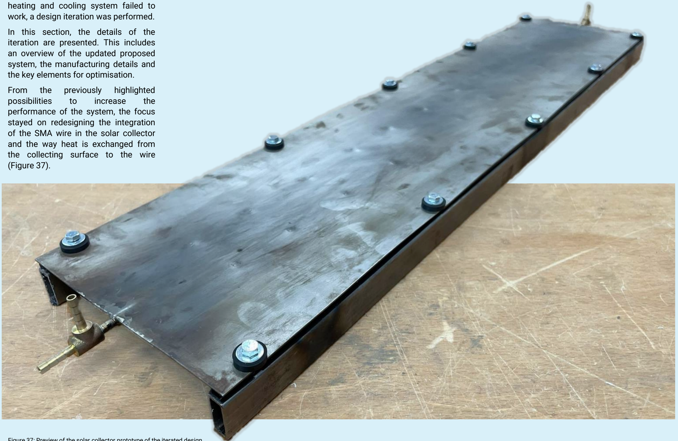
Figure 37: Preview of the solar collector prototype of the iterated design.
