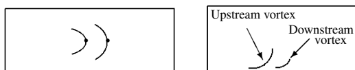
(a) Top view of two vortices aligned in streamwise direction. Distance between '••' is the streamwise spacing between two vortices given by \Delta x^+ . (b) Side view of two vortices with higher strength & higher y_e^+ upstream & lower strength & lower y_e^+ downstream, respectively. y_e^+ denotes y^+ value of reference plane for conditional eddy.
