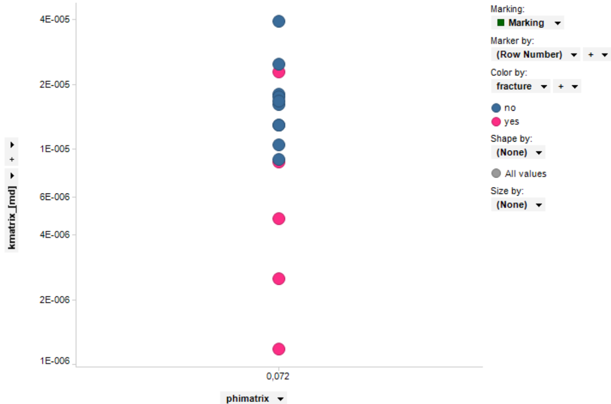
Figure 4.17: The effect of a high permeability streak on the matrix permeability on the sample EBN20.
