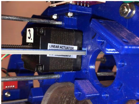
Figure 3.18: The slider, motor mounting plate and assembled motor are shown. An empty slot for an actuator is shown next to the mounted motor.
