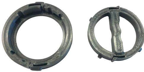
(a) Test print of connector. The proximal ring is shown left, the distal ring is shown right.
