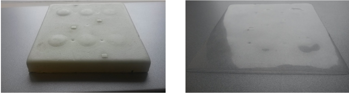
Figure D.2: The CNC'd Foam moulds (left) and finished product (right)
