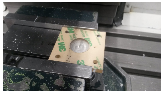
Milling a Pocket in the Manifold
