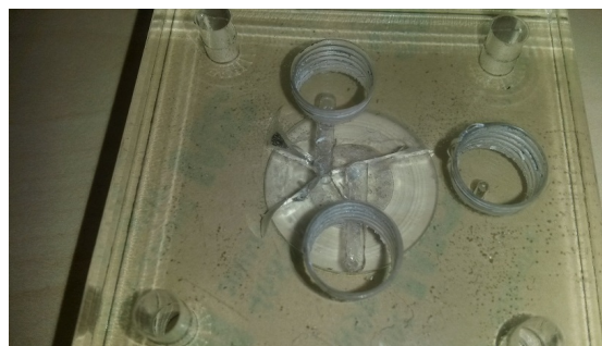
Figure D.8: Cracked PMMA Layer after Cleaning with Alcohol
