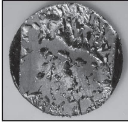
FIGURE 3.6 – Optical microscope image of a sample heated to 300 °C showing the peeling-off of the Pd cap layer.
