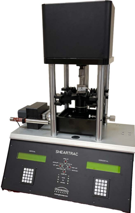
Figure 2.4: Cyclic Direct Simple Shear Test System - Source: Geocomp
