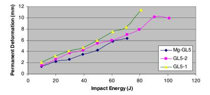
Fig. 9 Permanent deformations (maximum dent) for the tested laminates
