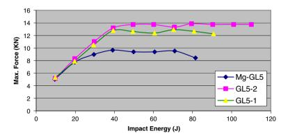
Fig. 5 Maximum impact forces for the tested laminates
