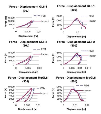
Fig. 12 Force-displacement curves, FEM and experimental results
