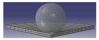
Fig. 1 Finite element model (mesh geometry). *Dark layers* are made of AL 2024-T3 or Mg AZ31B-H24 and *bright layers* are FM94/S2
