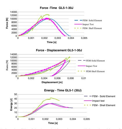
Fig. 13 Comparison of FE-predictions (energy-time) for two element types with the experimental data as reference
