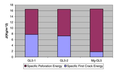
Fig. 4 Specific limit energies for the tested laminates
