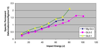
Fig. 10 Specific permanent deformations for the tested laminates
