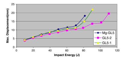
Fig. 7 Maximum displacements for the tested laminates
