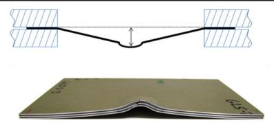
Fig. 8 The permanent deformation measurement
