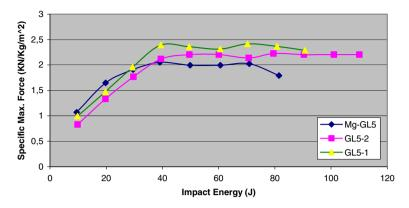
Fig. 6 Specific maximum force for the tested laminates
