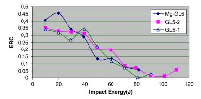
Fig. 3 ERC curves for the tested laminates
