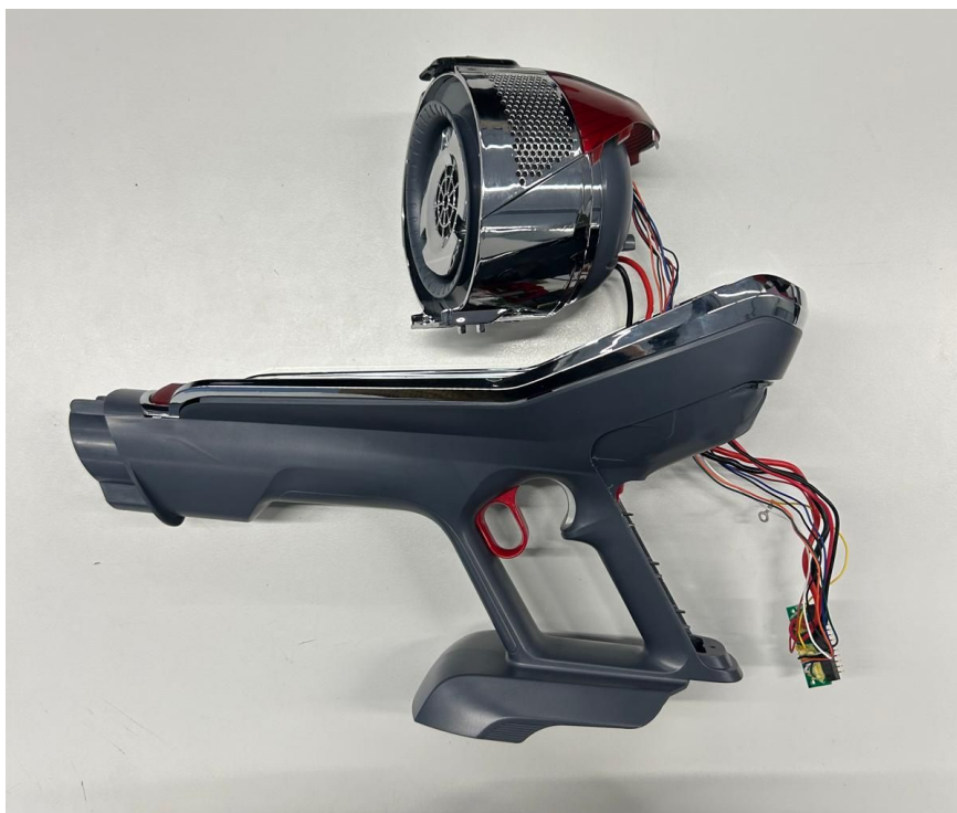
Figure 31. soldering cables to components limits accessibility
