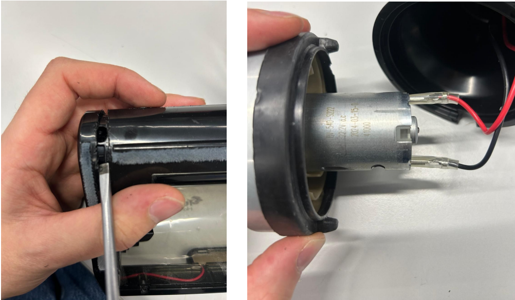
Figure 23. Hidden screw and easy to connect cable for the motor component
