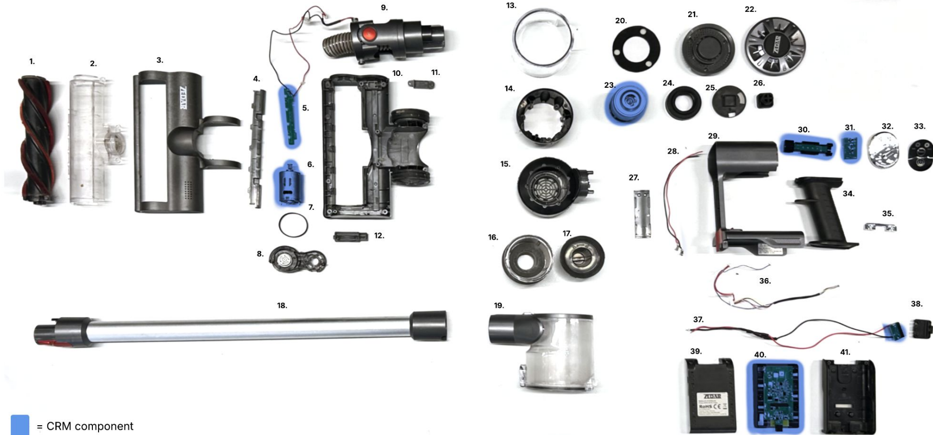
Knolled picture of Zedar S600 1. Brush; 2. See through cover; 3. Top head cover; 4. front head cover; 5. Lights PCB; 6. Brush motor; 7. Belt; 8. Motor converter; 9. Tube connector assy; 10. Bottom head cover; 11. Brush clip; 12. Spring clip; 13. See through motor cover; 14. Plastic motor cover; 15. Filter housing; 16. Outer filter; 17. Filter; 18. Tube; 19. Container; 20. Top motor foam; 21. Top motor cover; 22. Top housing cover; 23. Motor; 24. Motor rubber; 25. Motor PCB cover; 26. Rubber support; 27. Front housing plate; 28. connector cables; 29. Housing; 30. LEDs; 31. Control PCB; 32. Control end cap; 33. End cap cover sticker; 34. Handle; 35. Back plate; 36. Cable assy; 37. Power cable; 38. Power cable plate; 39. Battery top cover; 40. Battery + PCB; 41. Battery housing.
