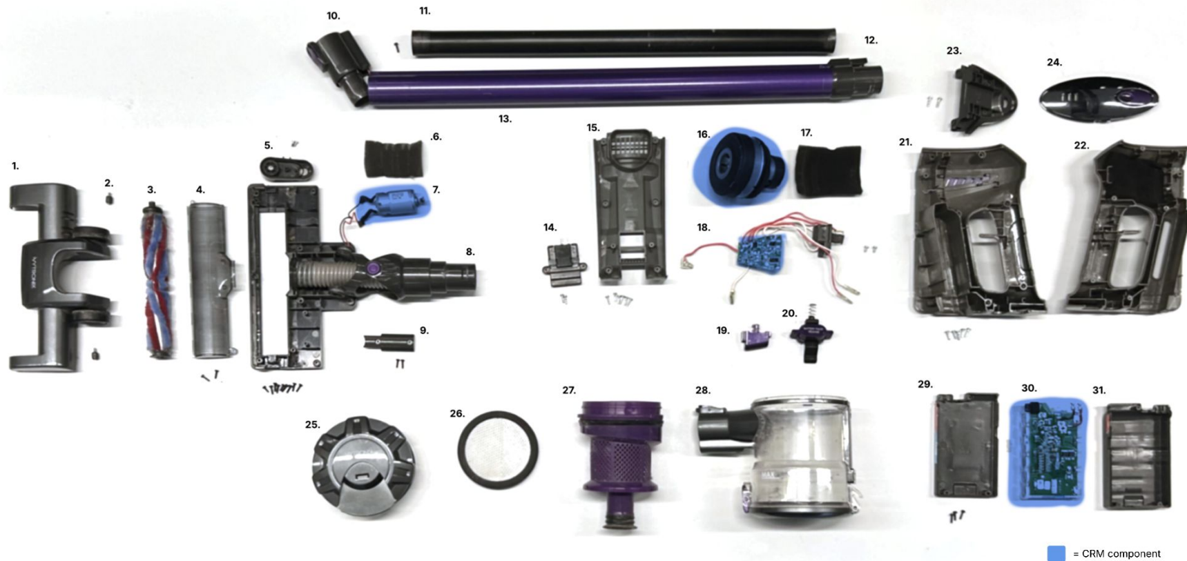
Knolled picture of Vytronix NIBC22 1. Head cover; 2. Wheel; 3. Brush; 4. See through cover; 5. Head side panel; 6. Foam cover; 7. Brush motor; 8. Bottom head assembly; 9. Cable cover; 10. Bottom tube connector; 11. Inner tube; 12. Top tube connector; 13. Outer tube; 14. Battery connector; 15. Front housing cover; 16. Motor; 17. Foam motor cover; 18. PCB assembly; 19. Trigger; 20. Battery release button; 21. Side housing R; 22. Side housing L; 23. Top housing cover; 24. Container release panel; 25. Top container assembly; 26. Filter; 27. Filter cover assembly; 28. Container housing; 29. Top battery cover; 30. Battery assembly; 31. Bottom battery assembly.
