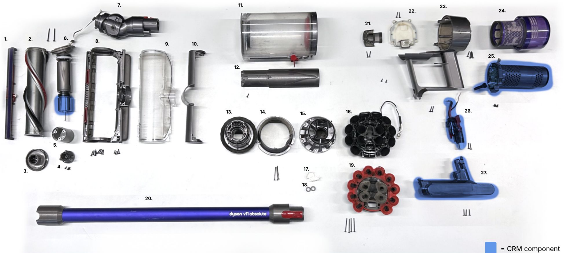
Knolled picture of Dyson V11 absolute 1. Front head cover; 2. Outer brush; 3. Brush end cap; 4. Motor top cover; 5. Motor side cover; 6. Inner brush assembly; 7. Head to tube assembly; 8. Outer head body; 9. See through cover; 10. top head cover; 11. Container; 12. Container rail; 13. Filter assembly top; 14. Filter assembly middle; 15. Filter assembly inside component; 16. Filter assembly bottom; 17. Cable cover; 18. Cable rings; 19. Filter assembly bottom cover; 20. Tube assembly; 21. Power cable cover; 22. PCB cover; 23. Handle; 24. Filter; 25. Motor + PCB assembly; 26. Trigger assembly; 27. Battery assembly.
