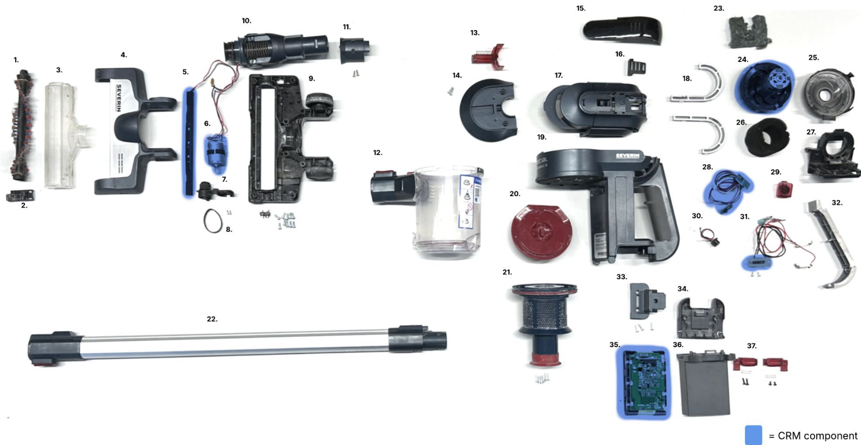
Knolled picture of Severin S Special 1. Brush; 2. Brush clip; 3. See through cover; 4. Top head cover; 5. LED; 6. Brush motor; 7. Motor converter; 8. Belt; 9. Bottom head cover; 10. Tube connector; 11. Tube connector cover; 12. Container; 13. Lid botton; 14. Lid; 15. Light panel; 16. Light diffuser; 17. Top housing; 18. Rails; 19. Main housing; 20. Filter cover; 21. Filter; 22. Tube; 23. Foam; 24. Motor; 25. Motor front cover; 26. Motor foam; 27. Motor cover front; 28. PCB Cable; 29. Power button; 30. Charger cable; 31. Battery cable assy; 32. Back panel; 33. Bottom panel; 34. Battery housing cover; 35. Battery + PCB; 36. Battery housing; 37. Battery connection buttons.
