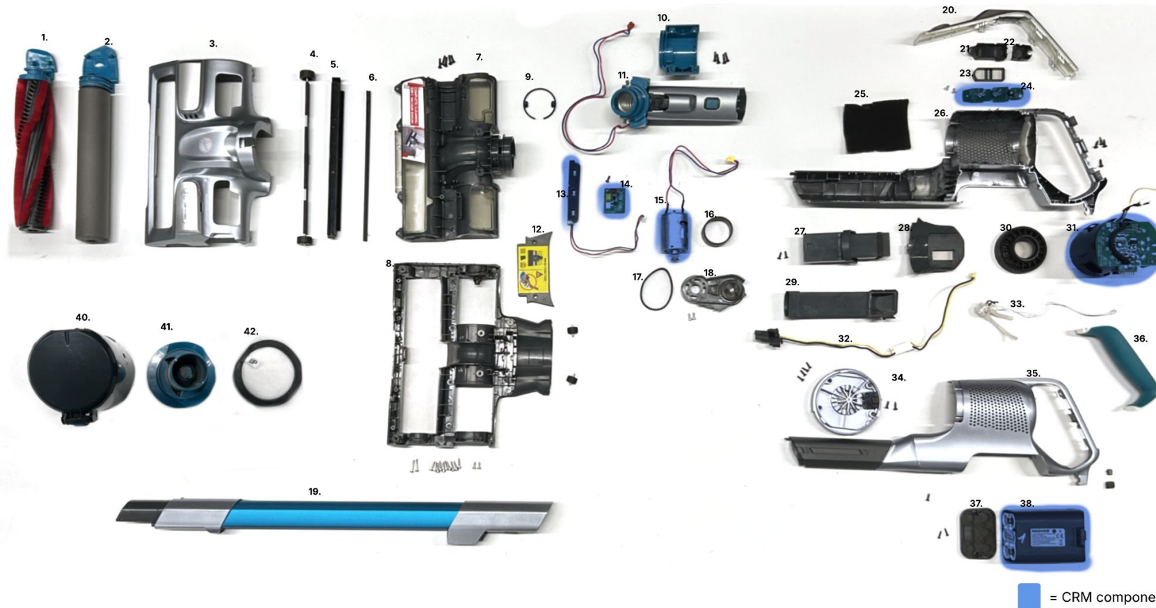
Knolled picture of Hoover H-Free 500 Hydro plus 1. Brush; 2. Roller; 3. Top head cover; 4. Front wheel assy; 5. Rubber guide; 6. Rubber guide guide; 7. See through cover; 8. Bottom head cover; 9. Connection ring; 10. Tube connector cover; 11. Tube connector; 12. Bottom head plate; 13. LED; 14. PCB; 15. Brush motor; 16. Motor rubber ring; 17. Belt; 18. Motor converter; 19. Tube; 20. Top housing cover; 21. Mode button; 22. Power button; 23. Button insert; 24. Button PCB; 25. Foam; 26. Housing L; 27. Tube connection; 28. Tube connection 2; 29. Tube connection 3; 30. Motor rubber cover; 31. Motor; 32. Power cable; 33. Cable assy; 34. Motor cover; 35. Housing R; 36. Handle; 37. Battery cover; 38. Battery housing + Battery; 39. Rubber; 40. Container; 41. Filter; 42. Filter top.
