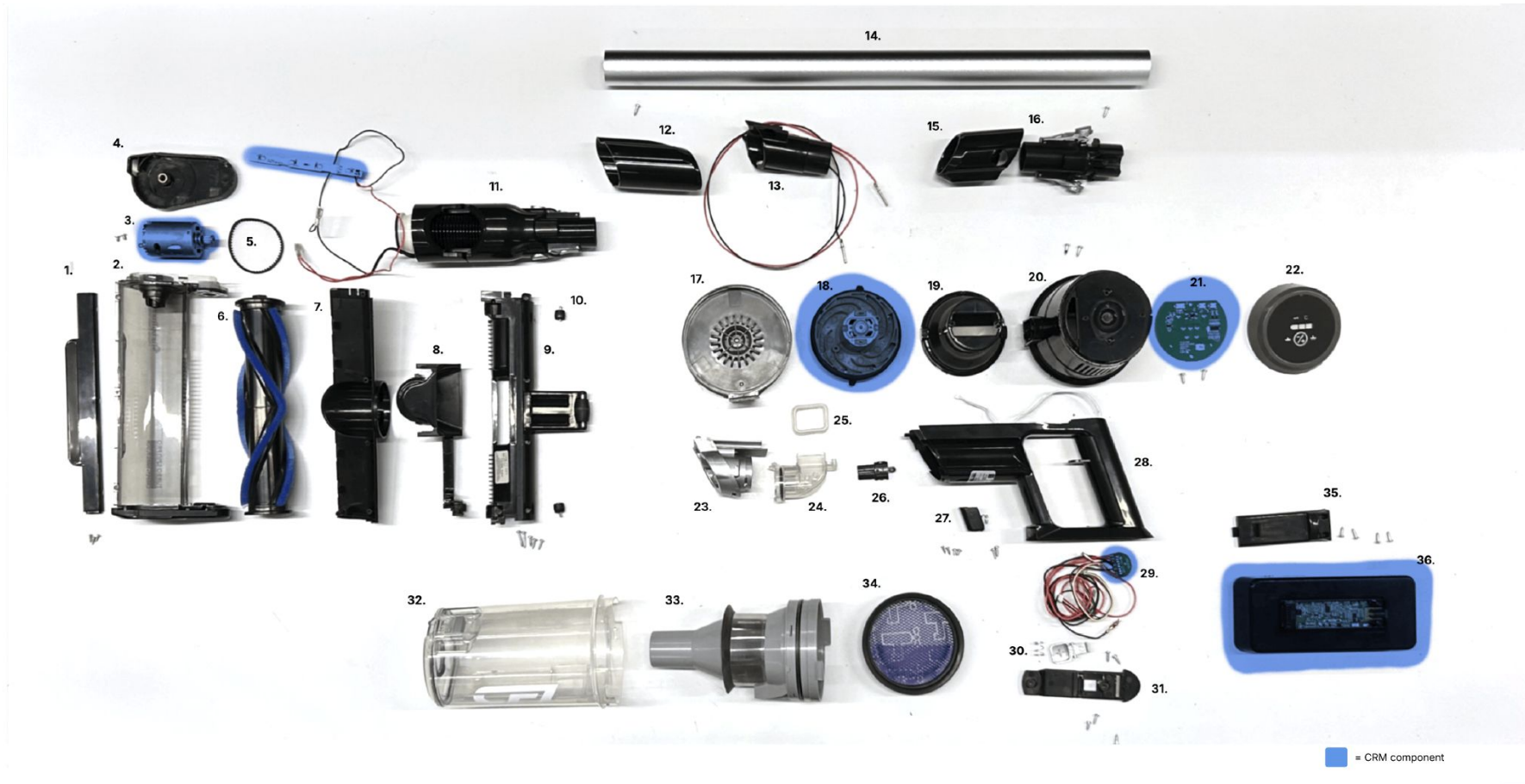
Knolled picture of TurboTronic TT-CF7 1. LED cover; 2. See through cover; 3. Brush motor; 4. Side panel L; 5. Motor belt; 6. Brush; 7. Top head cover; 8. Inner dust guide; 9. Bottom head cover; 10. wheels; 11. Head to tube assembly; 12. Bottom connector cover; 13. Bottom connector; 14. Tube; 15. Top connector cover; 16. Top connector; 17. Motor front cover; 18. Motor; 19. Motor housing; 20. Outing housing; 21. PCB; 22. Interface cap; 23. Container connector; 24. dust guide; 25. silicon ring; 26. Cable connector; 27. Trigger; 28. Controller handle; 29. cable assembly; 30. Battery release button; 31. Bottom housing cover; 32. Container; 33. Filter assembly; 34. Filter; 35. Battery cover; 36. Battery assembly.
