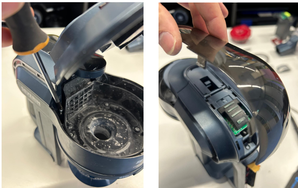
Figure 25. Hard to access screws and snap-fits
