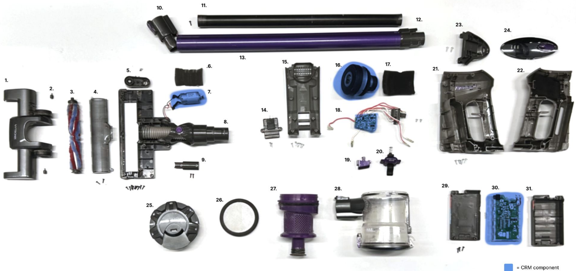
Figure 34. Knolled picture of Vytronix NIBC22 1. Head cover; 2. Wheel; 3. Brush; 4. See through cover; 5. Head side panel; 6. Foam cover; 7. Brush motor; 8. Bottom head assembly; 9. Cable cover; 10. Bottom tube connector; 11. Inner tube; 12. Top tube connector; 13. Outer tube; 14. Battery connector; 15. Front housing cover; 16. Motor; 17. Foam motor cover; 18. PCB assembly; 19. Trigger; 20. Battery release button; 21. Side housing R; 22. Side housing L; 23. Top housing cover; 24. Container release panel; 25. Top container assembly; 26. Filter; 27. Filter cover assembly; 28. Container housing; 29. Top battery cover; 30. Battery assembly; 31. Bottom battery assembly.
