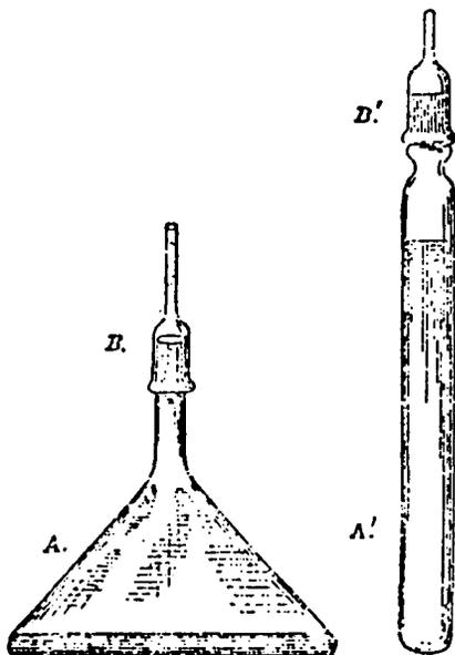
FIGURE 4. Examples of culture vessels used to produce "aerobic" and "anaerobic" conditions in early denitrification experiments (from Gayon & Dupetit, 1886).
