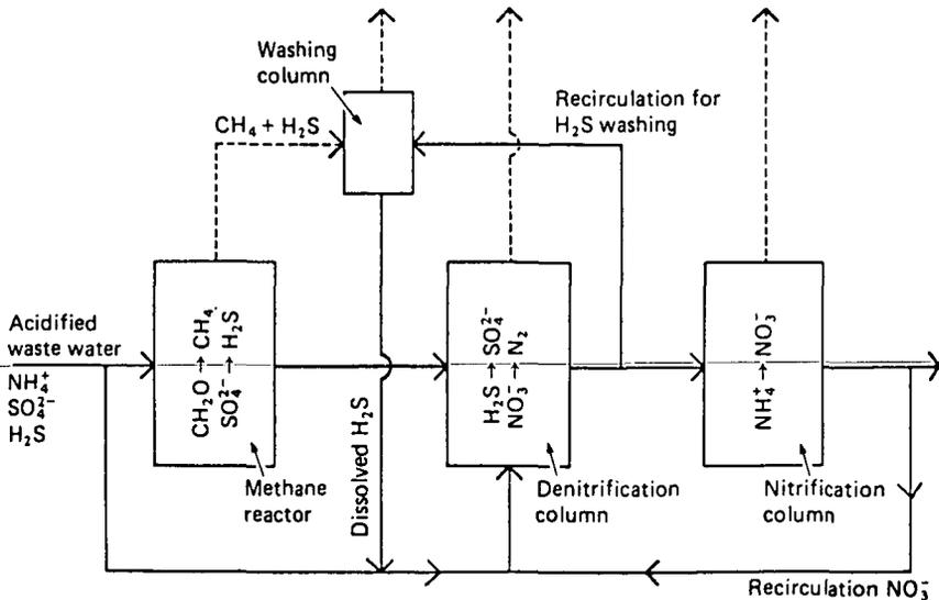
FIGURE 10. Outline of the sequential wastewater treatment system which includes the denitrification reactor under study.
