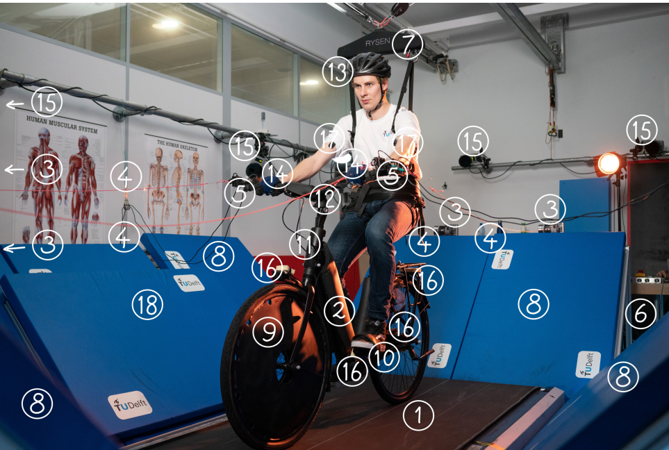
Figure 3.1: Overview of the experimental setup, with: 1-treadmill, 2-bicycle, 3-pull force motor (4), 4-pull rope (4), 5-force sensor (4), 6-Speedgoat real-time controller, 7-intelligent harness, 8-soft padding (8), 9-disc wheel cover (2), 10-foot strap (2), 11-mechanical rotation limiter, 12-rear-brake handle, 13-helmet, 14-protective gloves (2), 15-motion capture camera (12), 16-IMU (4), 17-EMG measurement unit (4), 18-folding fence.
