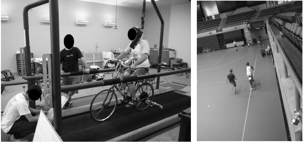
Figure 4.2: (a) A participant riding the instrumented bicycle on a horse treadmill. (b) A participant riding the instrumented bicycle in the indoor gymnasium. Both figures are adapted from Moore (2012) [38]. 2
