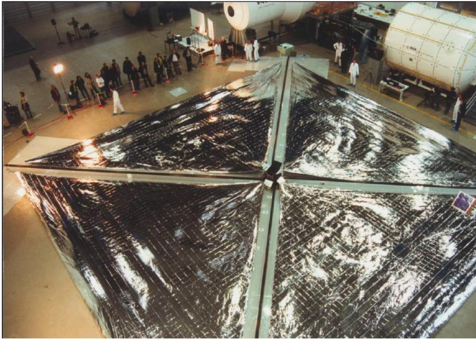
Figure 2.1: Solar Sail deployment test on ground at DLR [9].
