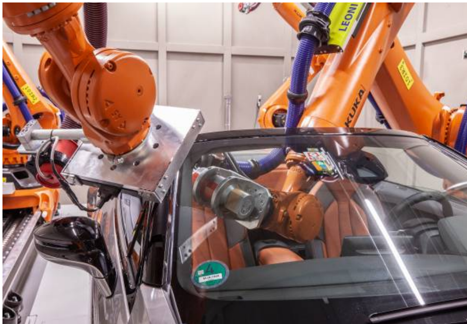
Figure 1-3: A robotic CT scanner for quality assurance developed by BMW [1, Figure 2]
