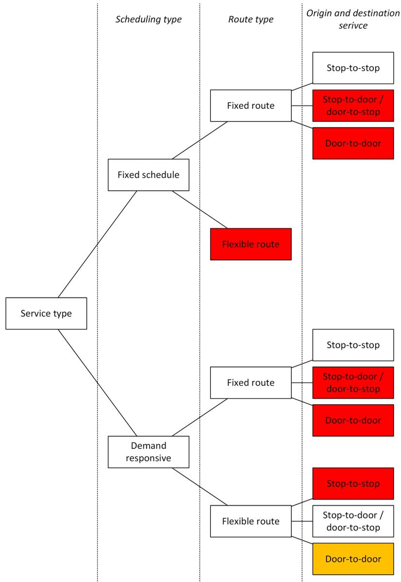
**Figure 2-7:** Service types for public transport, based on service type characteristics, from Table 2-3
