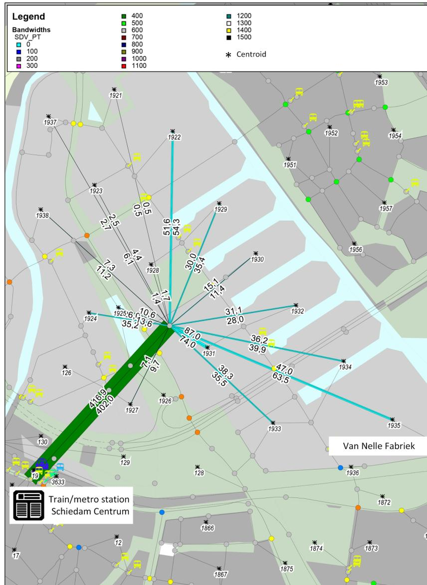
**Figure 5-1:** Number of trips (per direction, for the complete day) on the self-driving vehicle network for the test location Spaanse Polder & Van Nelle Fabriek
