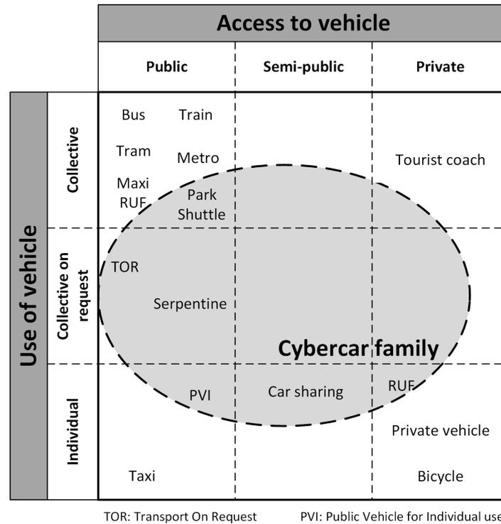
**Figure 2-9:** Classification according to access and use. Reprinted from [30]
