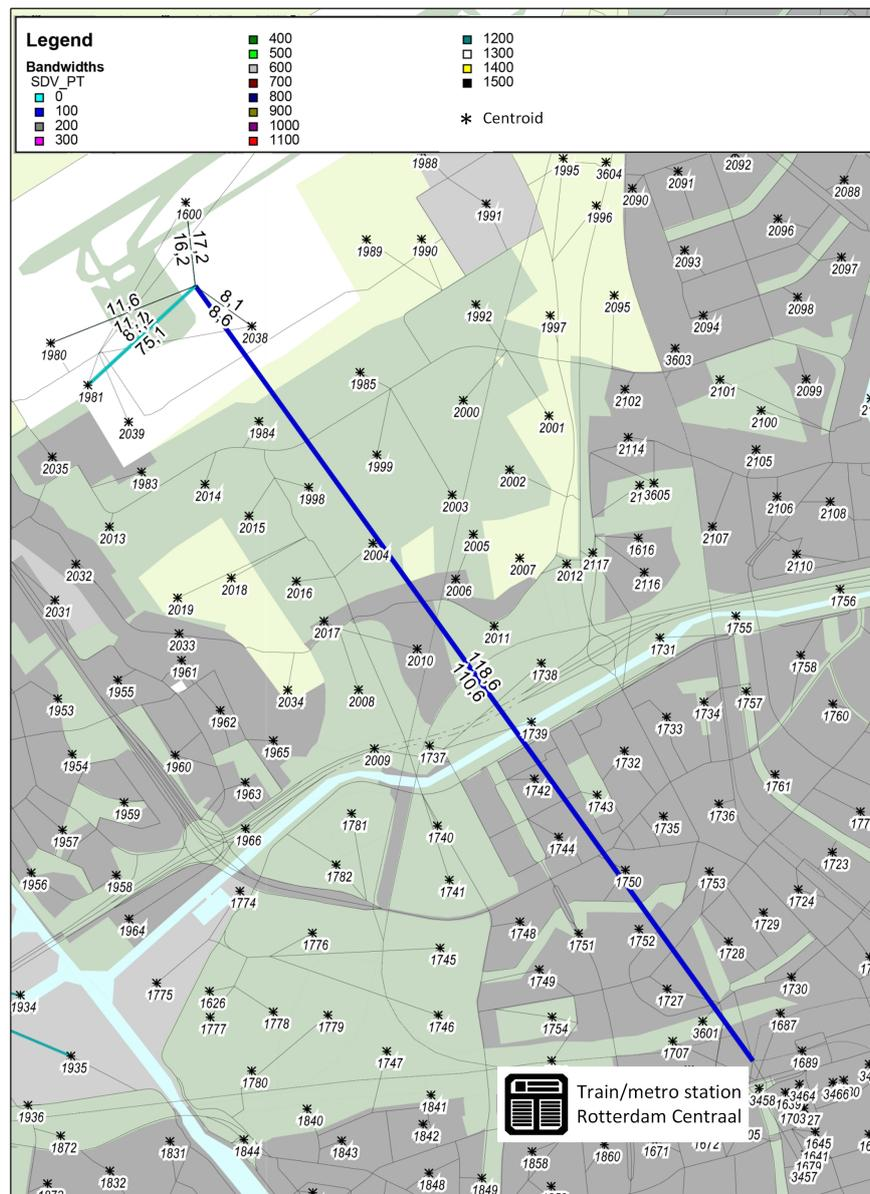
**Figure 5-2:** Number of trips (per direction, for the complete day) on the self-driving vehicle network for the test location Rotterdam The Hague Airport
