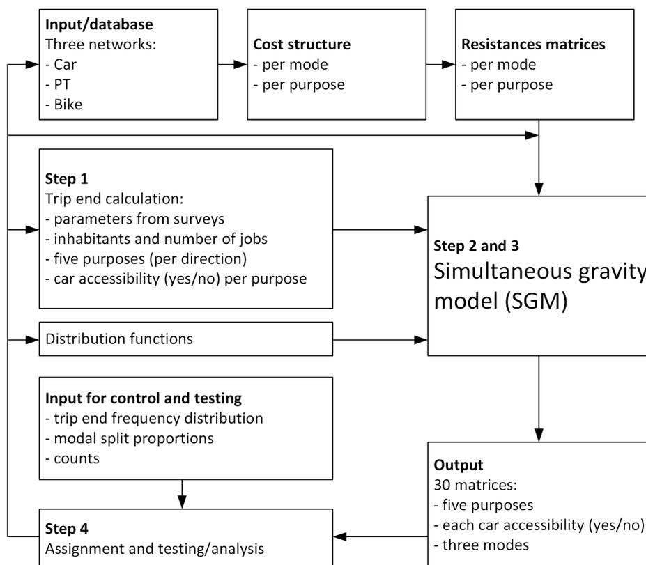
**Figure C-2:** Simultaneous gravity model (SGM) RVMK3.0. Reprinted from [78]
