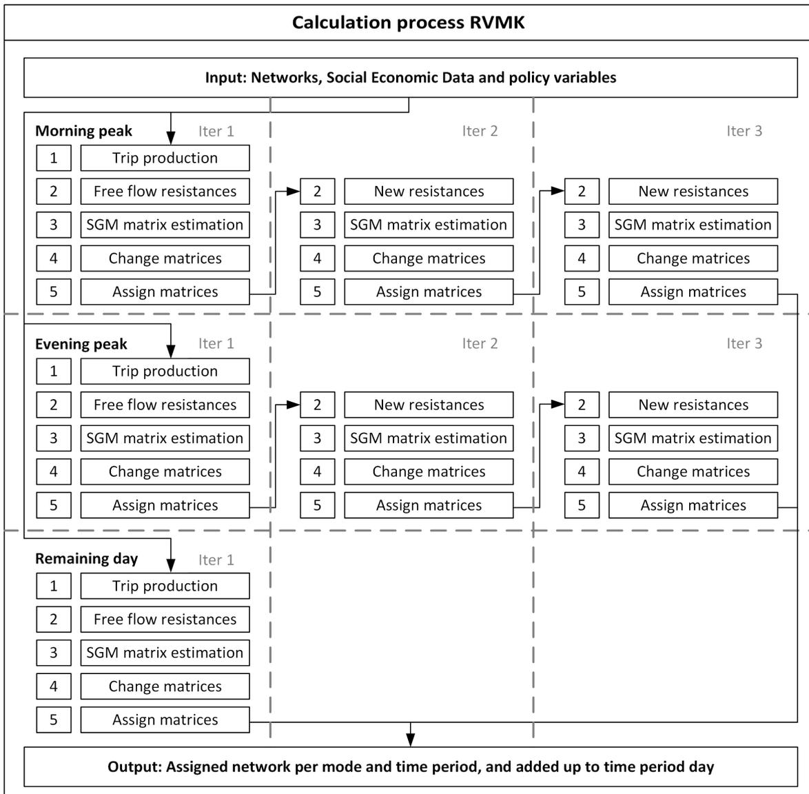
Figure C-3: Calculation process RVMK3.0. Reprinted from [78]
