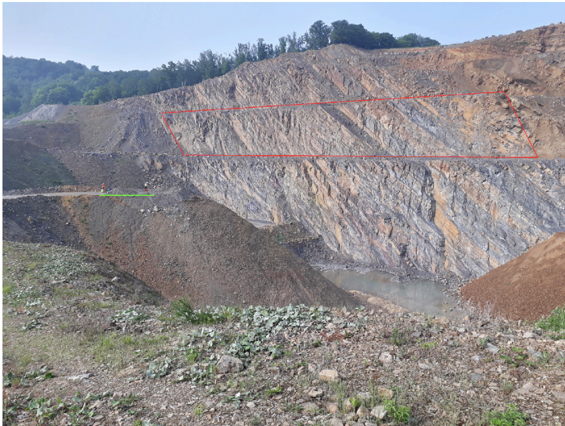
Figure 3.41: The Condroz sandstone outcrop in Trooz, for scale and scanning position you may notice the scanner setup in centre left of the picture. With the main outcrop segment highlighted in red and scanning platform underlined in green.
