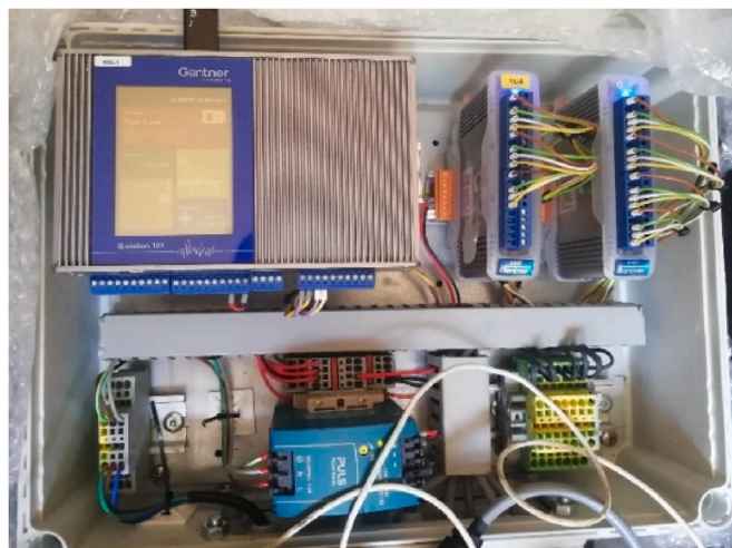
Fig. 18. DAQs of XPM10 pressure sensors.
