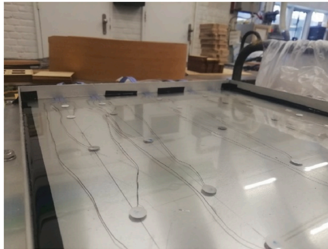
Fig. 11. Fully cured retrofit sensor layer.
