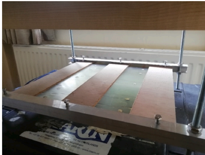
Fig. 22. Three bands composite support plate.
