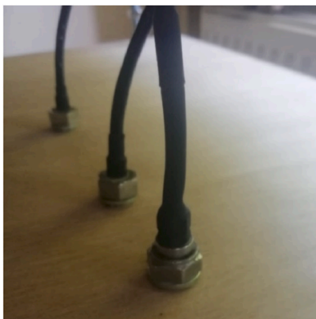
Fig. 19. Three XPM10 bolted to the mounting plate.
