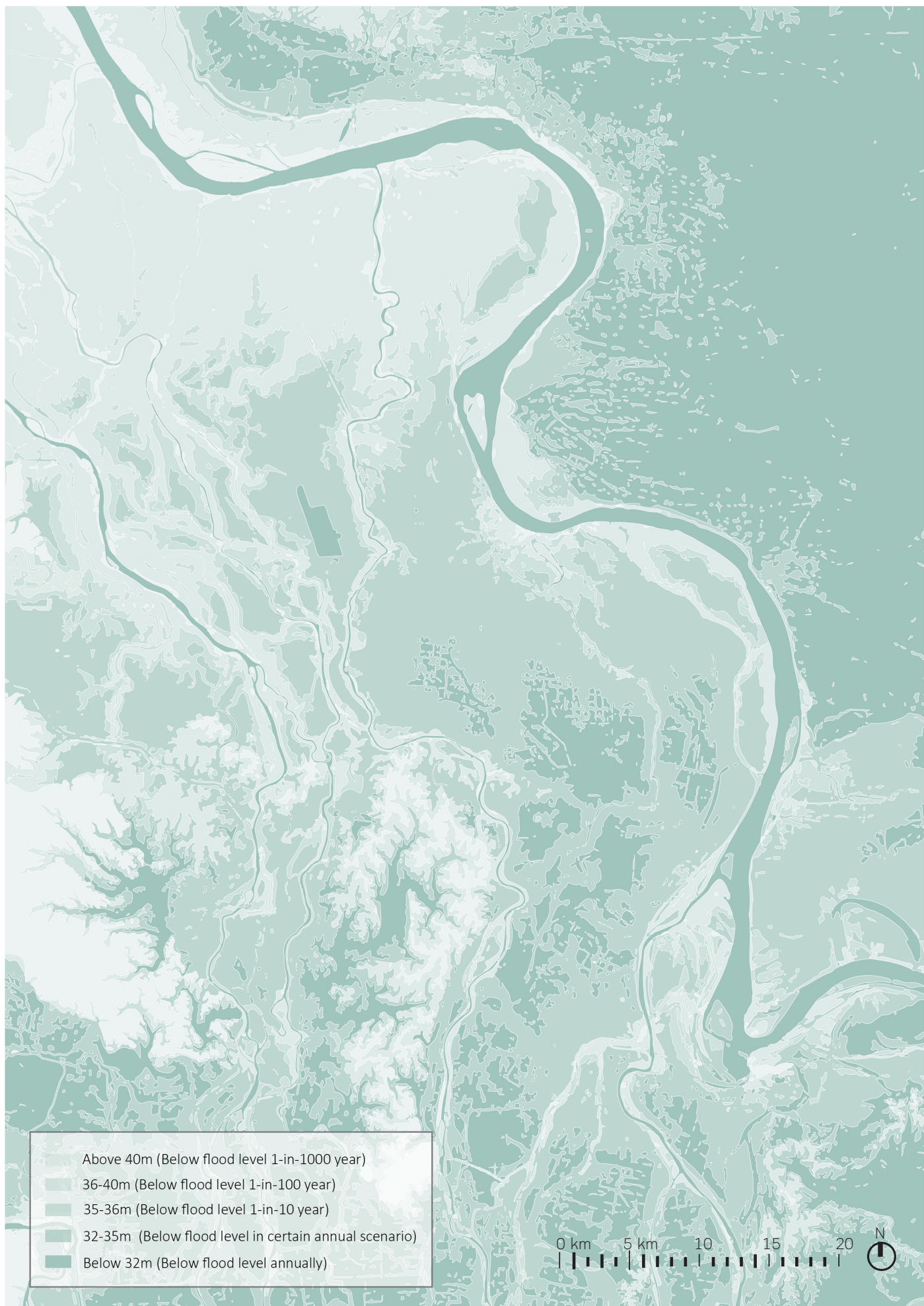
Fig.3.4. Terrain level according to flood scenario
