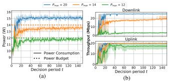
Fig. 8: Convergence rate evaluation of SBP-vRAN for different values of the power budget  $P_{\text{max}}$ .
