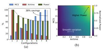
Fig. 3: (a): 8 combinations of normalized MCS and airtime providing 2.6Mbps in UL, and its associated power (idle mode power is subtracted). (b): Normalized power consumption at the BBU over baseline for full buffer UL transmissions and high SNR, as a function of MCS and airtime.
