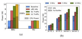
Fig. 1: (a): Comparison of power consumption at: the BBU (Intel NUC i7-8559U@2.70GHz), the BBU's CPU, and the RU (an USRP SDR), with 20Mbps DL and UL traffic. (b): Consumed power over the baseline for different radio bandwidths and hardware platforms. SF PC 1: Intel NUC i7-8559U@2.70GHz; SF PC 2: Intel NUC i7-8650U@1.90GHz; Server 1: Dell XPS 8900 i7-6700@3.40GHz; Server 2: Dell Aurora R5 i7-9700@3.00GHz.
