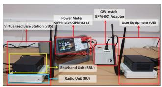
Fig. 6: Experimental vBS and UE testbed.
