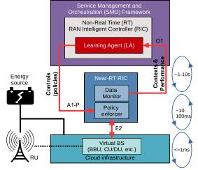
Fig. 5: O-RAN compliant system architecture and workflow.
