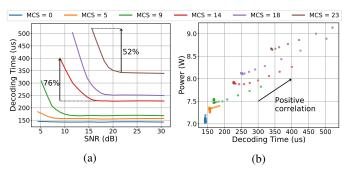
Fig. 2: vBS over SF PC 1 at full UL buffer. (a): UL decoding time as a function of SNR and different MCS values. (b): Power consumption as a function of the decoder performance (high correlation).
