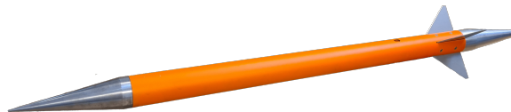
Figure 3.1: The DART XL Dart, an unpropelled payload stage. [Source: T-Minus Engineering archive]
