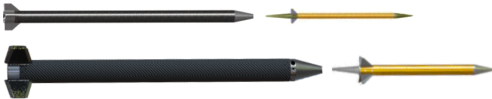
Figure 2.2: The T-Minus DART and DART XL vehicles, with the booster in black and the payload compartment in orange. [Source: T-Minus Engineering archive]
