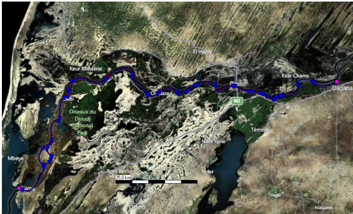
Figure 5-1: Modelled river stretch of the system area between Dagana and Diama. The boundaries, profiles and calculation points are indicated in pink, blue and red respectively.
