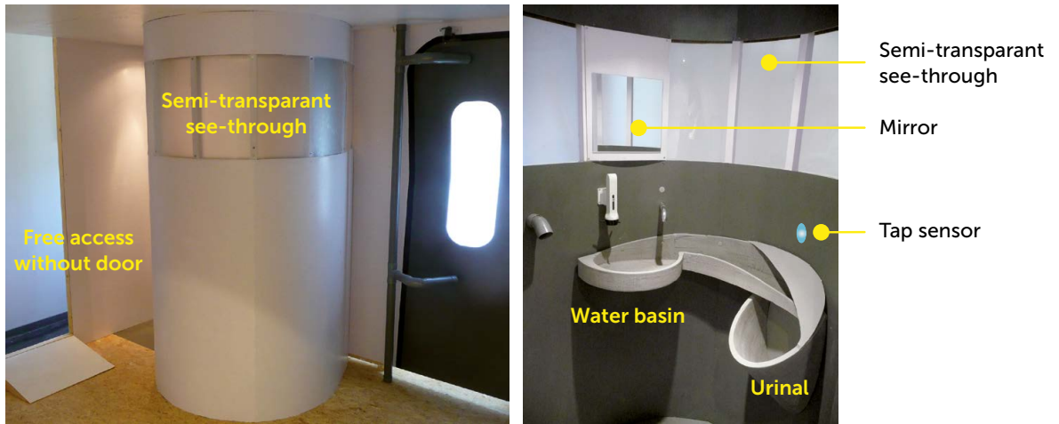
Figure 7.6a. exterior and 7.6b Interior of mock-up 1: urinal module
