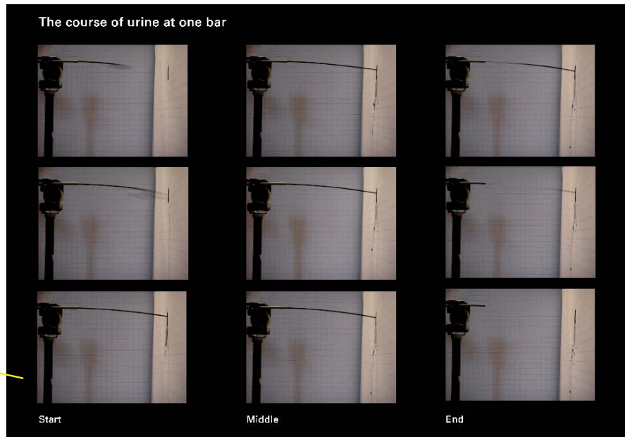
Figure 6.18d Side view dispersion test 1 bar
