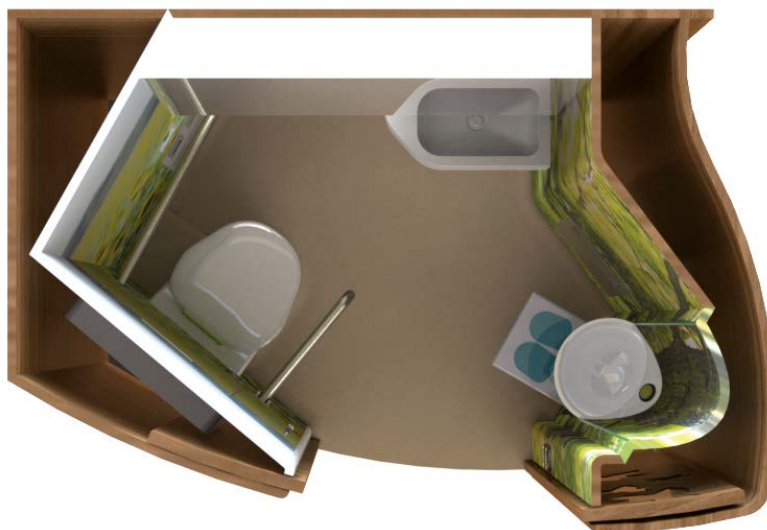
Figure 8.3 Lay-out train toilet, urinal is hidden in a recess Rendering: Tommy Louts and Fleur Derks
