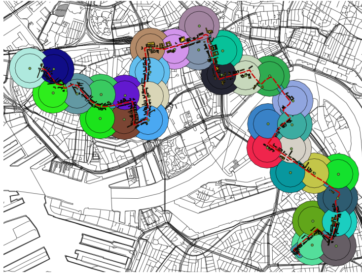
Figure 5.9: A top-down display of the the collision spheres used for loading information in the game engine. The larger of the two sphere is the one triggering the loading of a tile, while the smaller triggers its visualisation.
