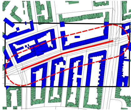
(a) The result of the bounding boxes intersection: the blue footprints intersect the bufer's bounding box.
