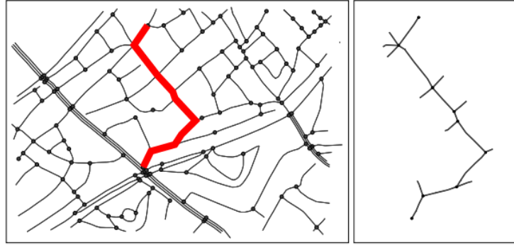
Figure 3.1: Left: bold line represents a “conventional” shortest-path visualisation. Right: The Choreme map representation of the same route. (Klippel et al., 2006)
