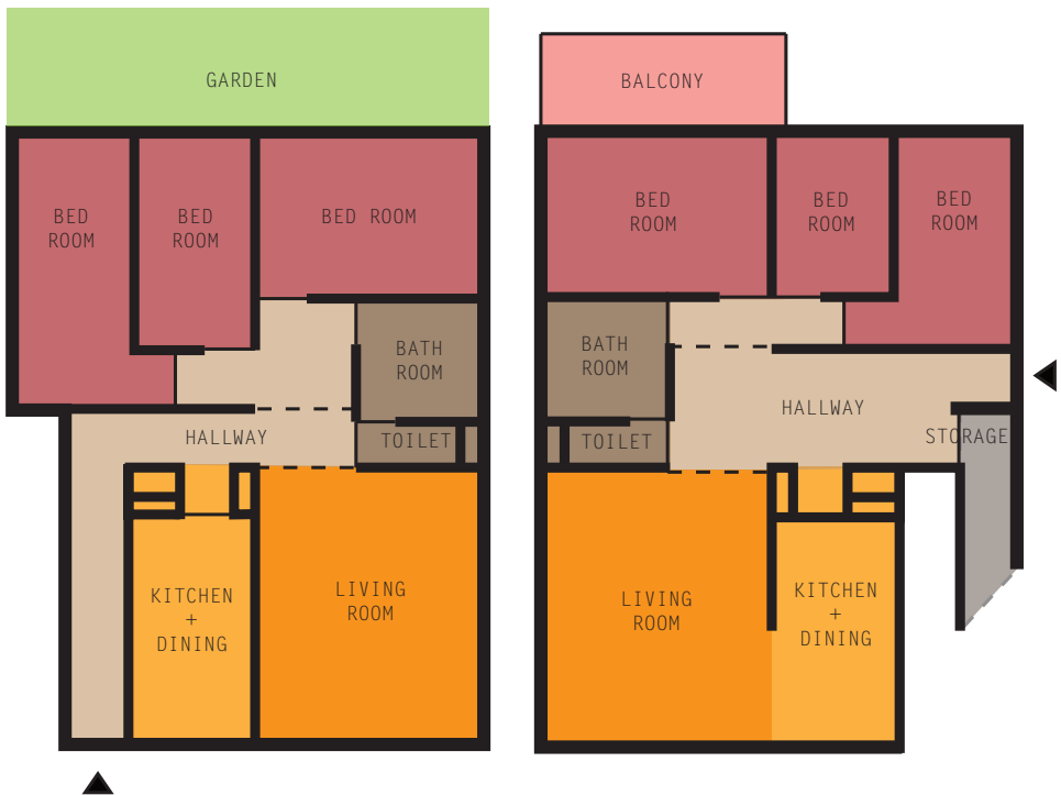
APARTMENT TYPE WITH AND WITHOUT BALCONY (LEFT GROUND FLOOR; RIGHT FIRST FLOOR)
