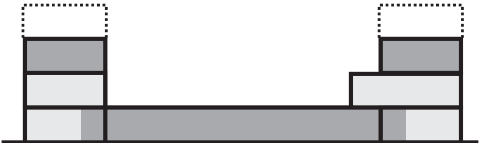
SEPARATION OF PUBLIC AND PRIVATE SPACE IN THE DWELLING IN FLOOR PLAN AND SECTION
