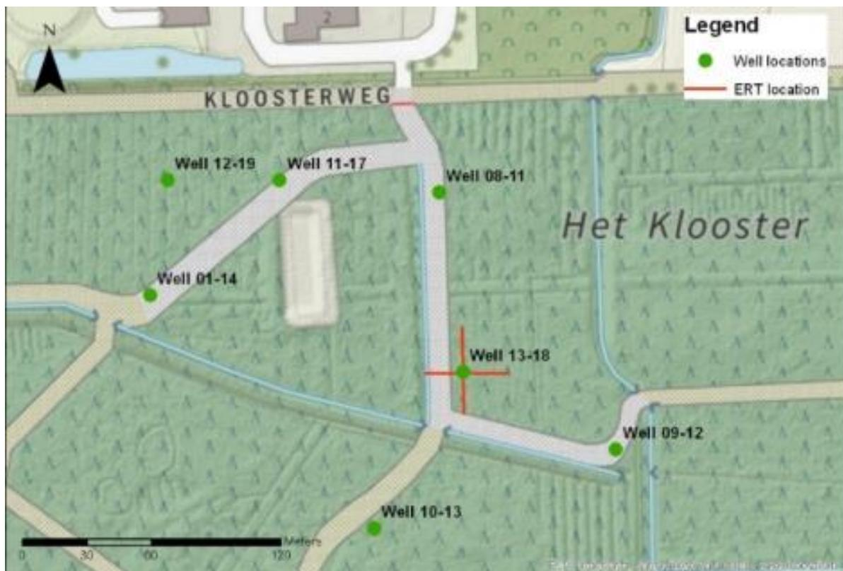
Figure 4: Image of well field 't Klooster. The red cross shows the location where time lapse ERT was performed. From: Karaoulis et al. (2019)
