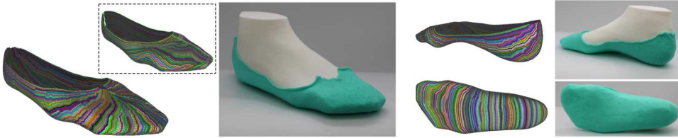
Figure 3.20: The sock example can be seamlessly fabricated by digital knitting using the stitch mesh (left) generated by our field-based optimization approach. The knitting result (right) perfectly fits the input shape of the feet which is 3D printed. The stitch mesh circled by dash-lines is a result generated by only using short-row shaping – therefore an additional seam is needed.
