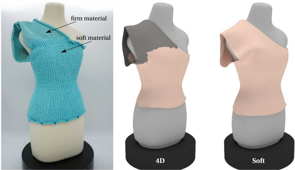
Figure 4.9: One-shoulder knitted top with prescribed material distribution to achieve a desired shape. Firm material on the shoulder produces a stiff style, while soft material on the torso ensures comfort. From the simulation, it can be found that the style cannot be achieved using a uniformly soft material.
