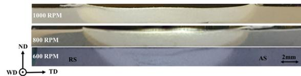
**Fig. 2.** Macrostructure of the cross-sections transverse to the welding direction at various rotational speeds (RS: retreating side, AS: advancing side).
