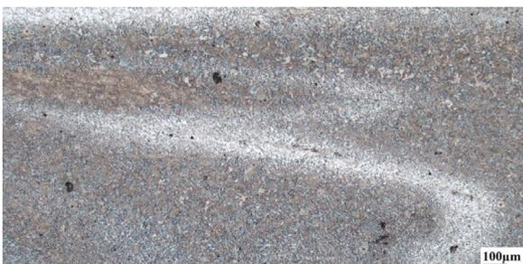
Fig. 9. Formation of a band of ferrite in SZ at tool rotational speed of 600 rpm.
