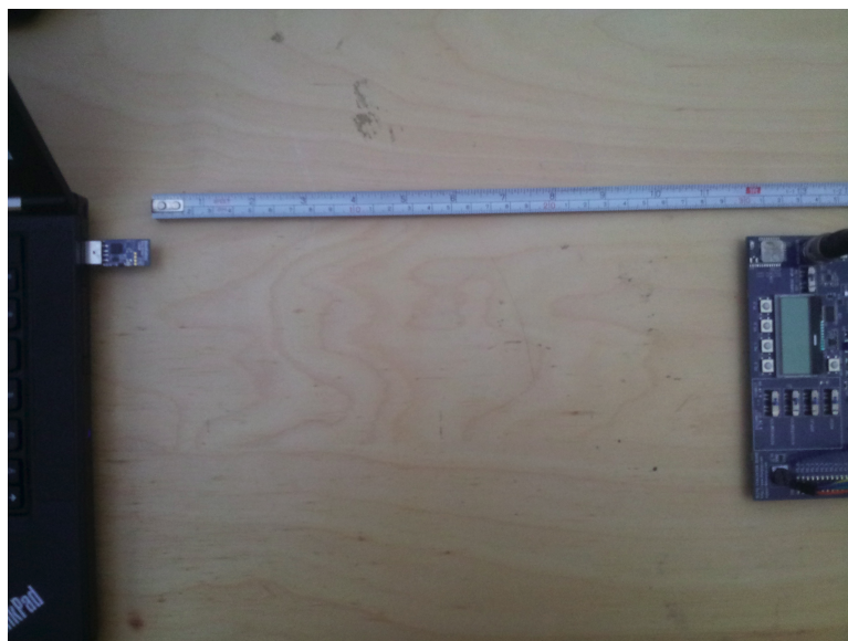
Figure 4.3: Overview of distance between radios of 30cm end to end. The radios are about 4mm further apart.
