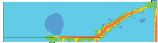
Figure 16.11 Crack pattern smooth reinforcement,  $u=700mm$
