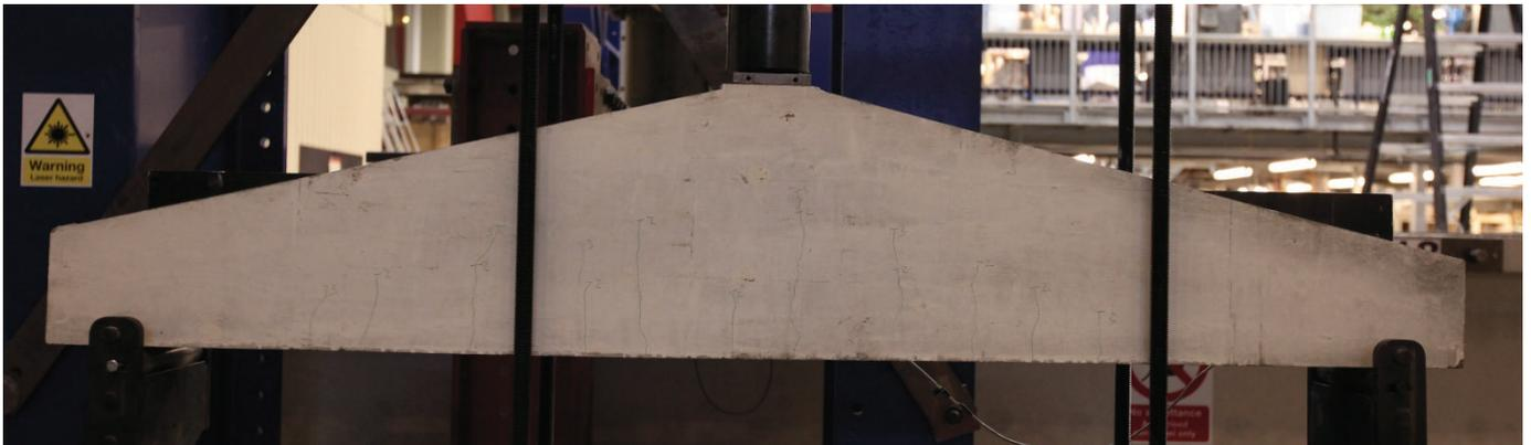
Figure 16.18 Bending cracks descending beam
