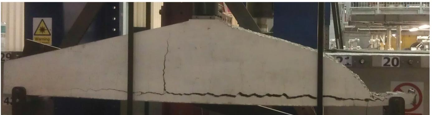
Figure 16.19 Descending beam after failure
