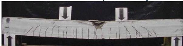
Figure 14.2 Crack pattern 4 point loaded beam (Sumajouw and Rangan, 2006)
