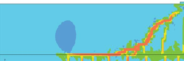
Figure 16.4 Crack pattern with extra reinforcement
