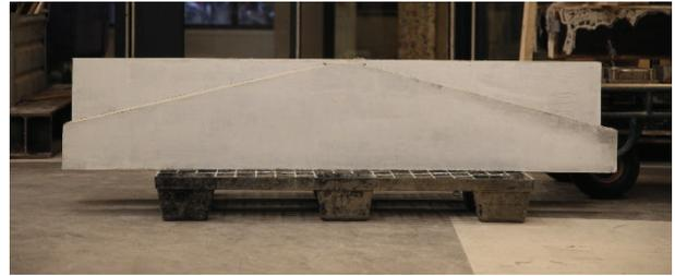
Figure 16.16 Beam and descending beam before testing
