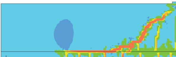
Figure 16.4 Crack pattern with extra reinforcement
