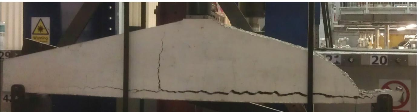
Figure 16.19 Descending beam after failure
