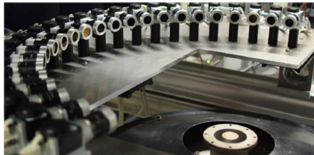
Figure 3.6: CTC setup constituting 24 CCD cameras with filters arranged around the swirl burner. Adopted from Mohri et al. [20].
