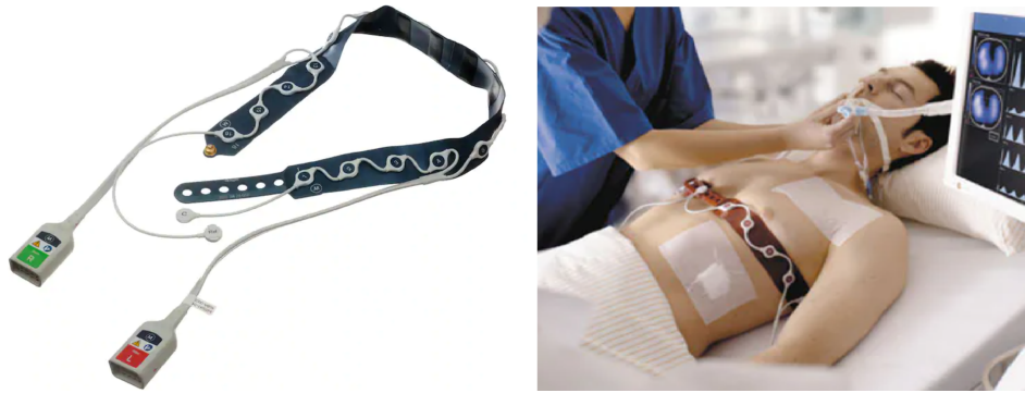
Figure 2.1: Left image: example EIT belt. Right image: patient wearing the EIT belt around the thorax. Images from Draeger ( www.draeger.com/Library/Content/EIT-Mini-Manual.pdf )
