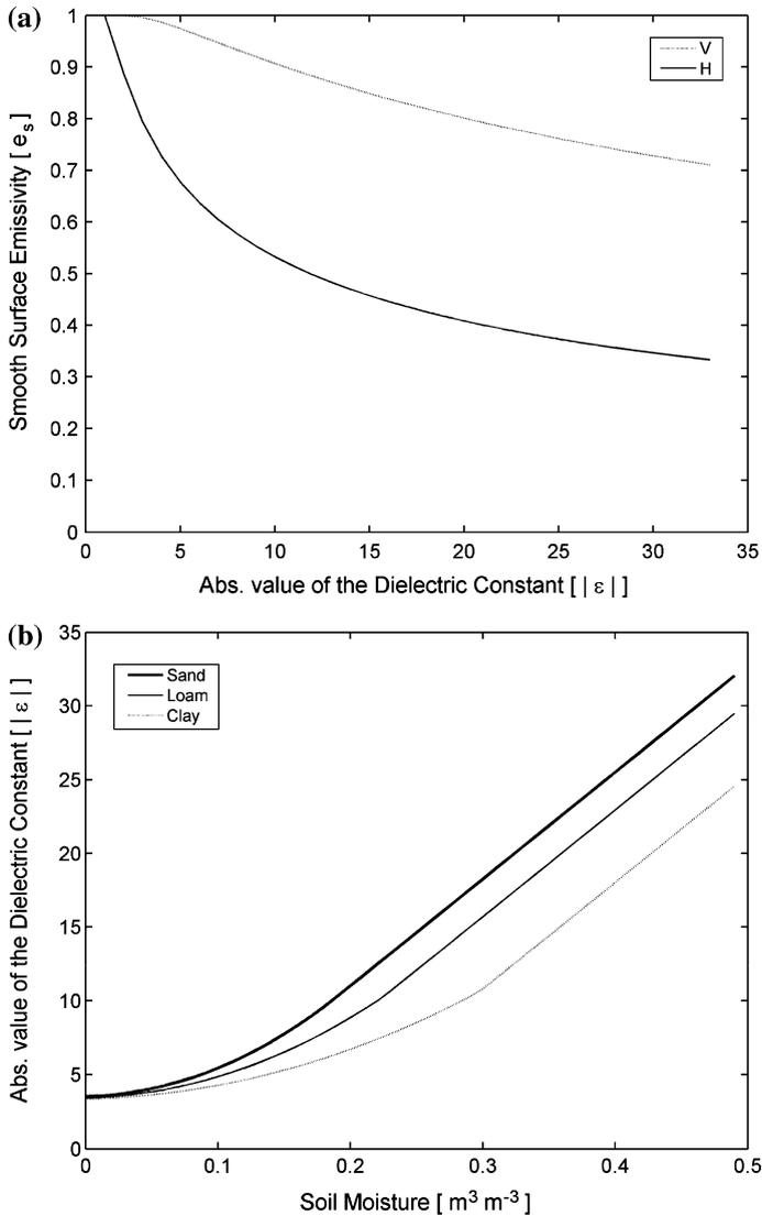
**Fig. 1** (a) Comparison of smooth surface emissivity and the soil dielectric constant according to the Fresnel relations with an incidence angle of 55 degrees. (b) Comparison of the soil dielectric constant and soil moisture for typical sand, loam and clay soils
