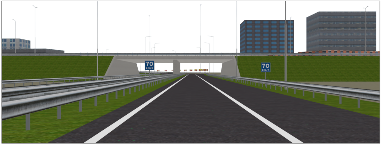
Figure 9: The announcement of the single-lane small-radius connector road with an advisory speed limit
