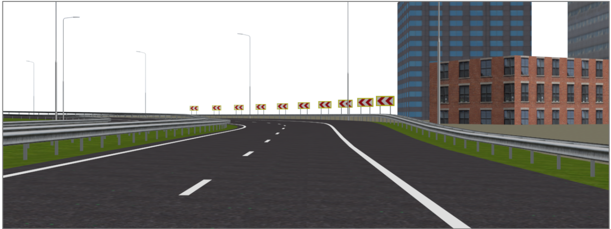
Figure 12: The signs in the shoulder lane of the mainline roadway, which warn for the small-radius curve
