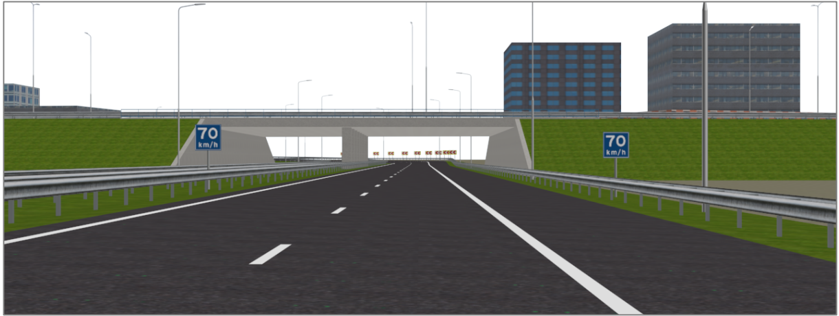
Figure 11: The announcement of the two-lane small-radius connector road with an advisory speed limit
