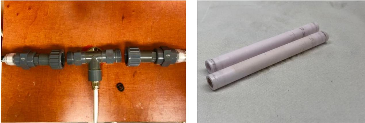
Figure 3.2: PVC membrane housing with rubber bearings (left) and Membrane T03 and T09 (right)
