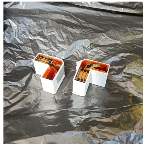
(b) Filling compartment with epoxy.
