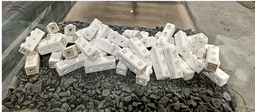
Figure 3.14: Setup with randomly placed blocks.
