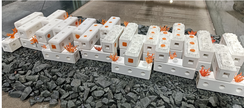
Figure 3.13: Setup 8, two top block variations and marine growth. Rounded top blocks on the left, additional roughness top blocks on the right.
