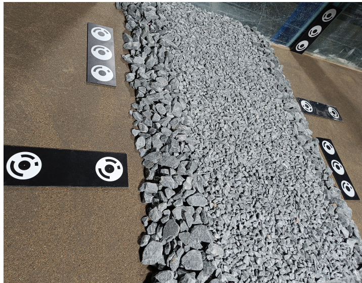
Figure 3.16: Photo of the underlayer with surrounding markers plates.
