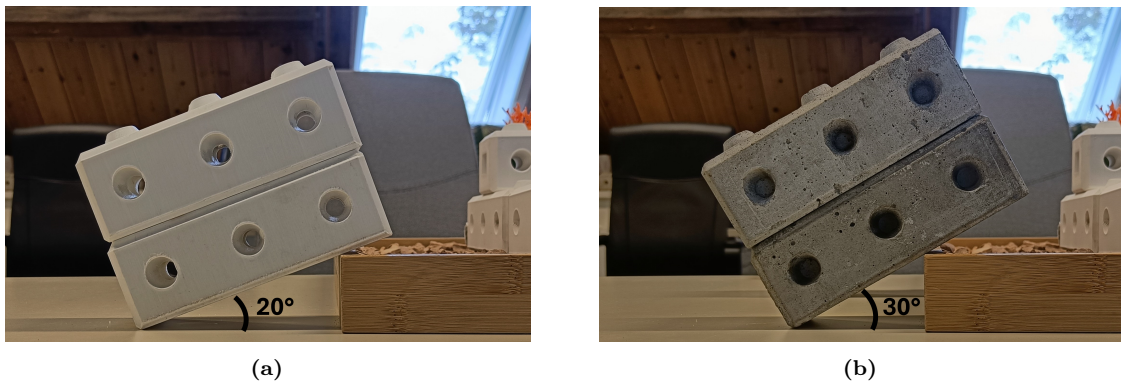
Figure 6.2: Maximum achievable angle of repose for PLA (a) and concrete (b) blocks.
